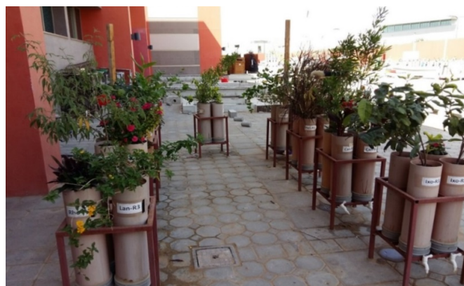
Figure 2 The 36 biofiltration columns.
