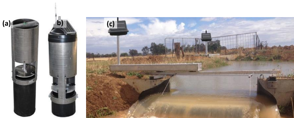
Figure 5-24 – Components of the AWMA on farm automation system (AWMA) (a) I-RiserPLUS, (b) I-RiserPLUS with removable control node, (c) I-Lifter flap gate (AWMA)
