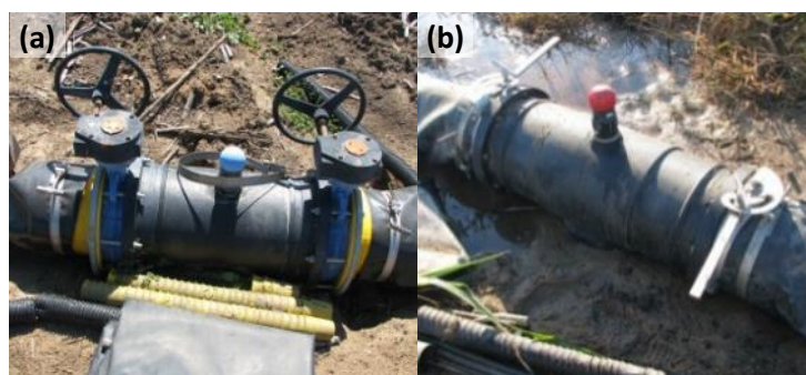
Figure 5-5 – Examples of butterfly valves currently used by farmers: (a) T fitting with two geared butterfly valves, (b) T fitting with two lever action valves.
