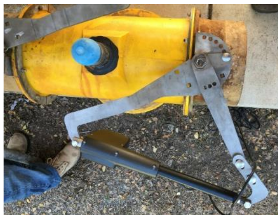
Figure 6-2 - Valve actuator lever prototype
