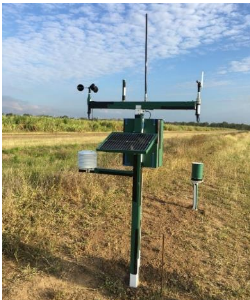
Figure 9-9 – Weather station installed at Jordan site.
