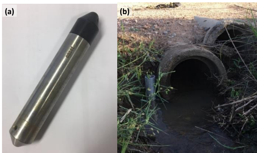
Figure 6-26 – HOBO PST (a) and installed in drain next to culvert for blocks 1-4 (b)
