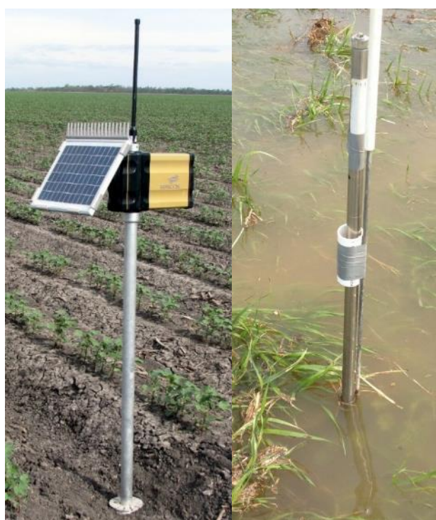
Figure 5-30 – (a) Rubicon Floodtech sensor node (b) Intech WT-HR capacitance probe
