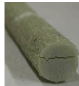
(c) Failure of #8 bars
