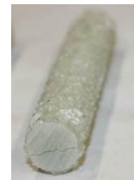
(b) Failure of #3 bars
