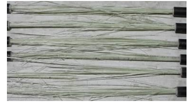
(b) Failure of #3 bars
