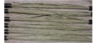
(c) Failure of #8 bars
