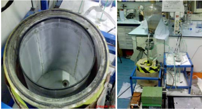
Figure 2. Inside view of the Hydrolytic Reactor (HR) without the stirrer (left). Photo of the laboratory HR set-up (Right).
