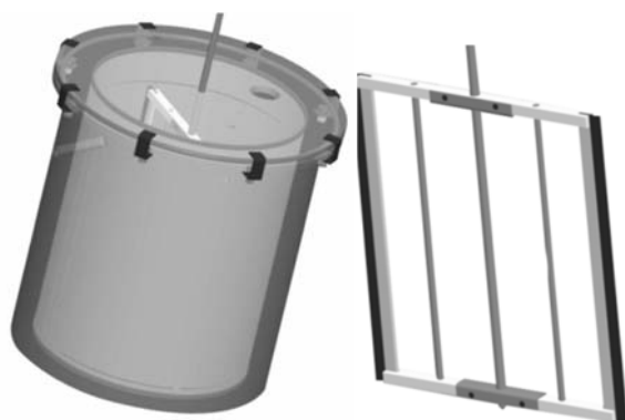
Figure 1. 3-D view of the hydrolytic reactor (left) and stirrer (right).
