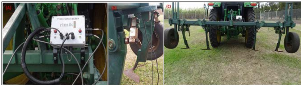
Figure 3. Overview of the experimental tillage unit used in the study, (A): Close-up of data-logger, (B): Close-up of the force transducer, and (C): Plan view of tractor and tillage unit.
