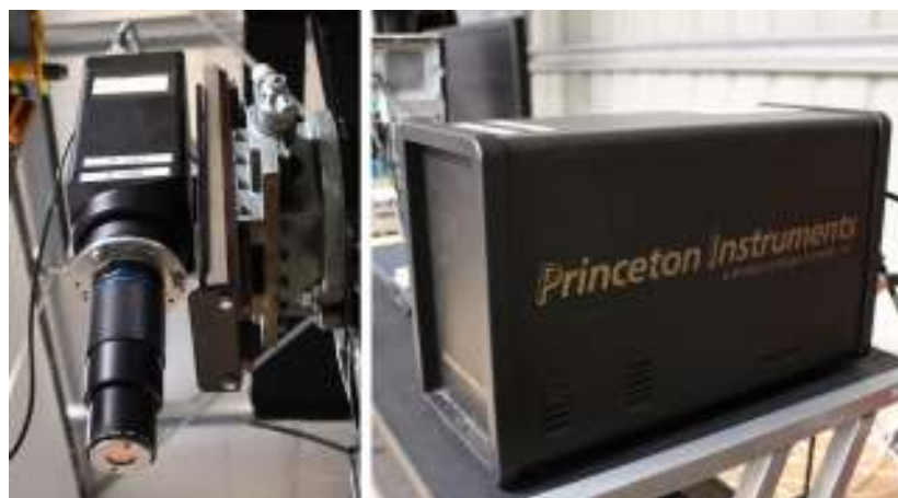
Figure 3.65: ICCD camera setup for \text{OH}^* chemiluminescence measurement.
