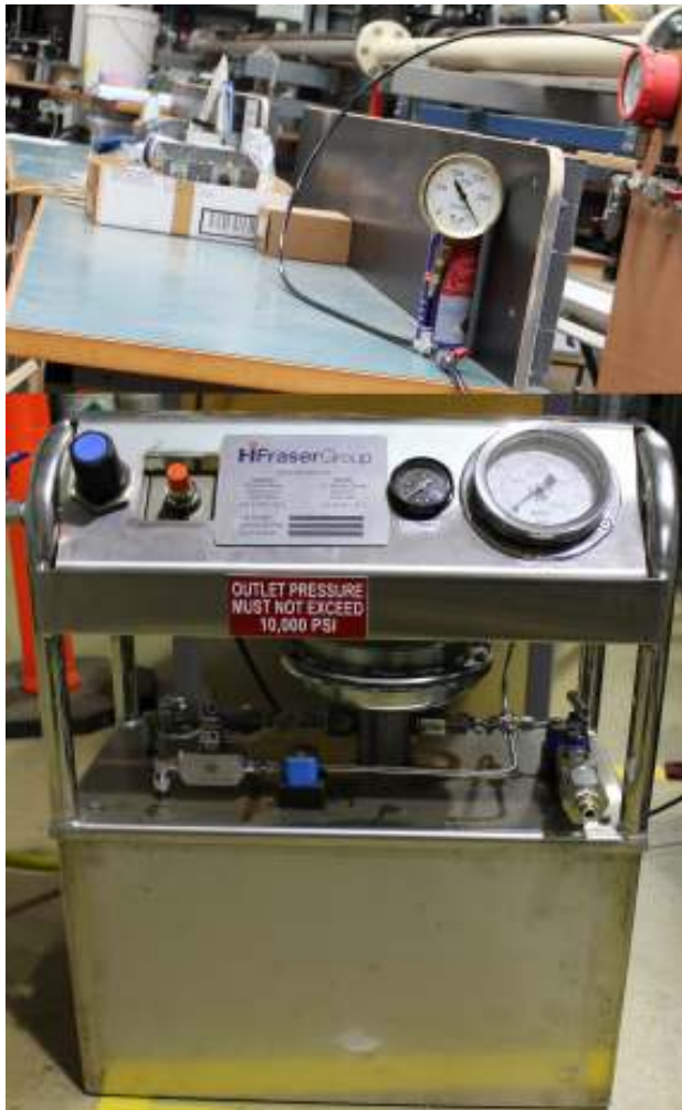
Figure 3.41: Photograph of the hydraulic device used for pressure testing.
