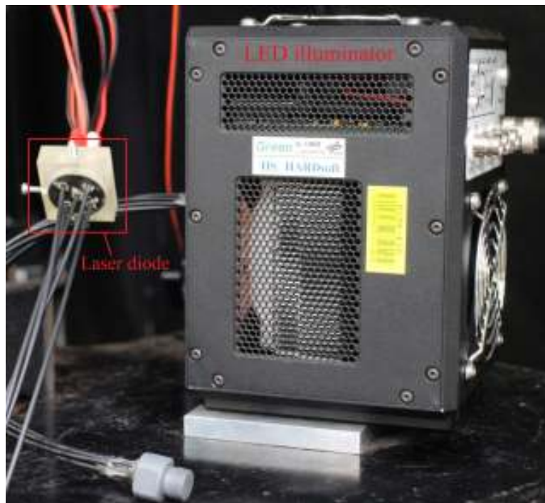
Figure 3.63: Photograph of light sources: LED illuminator and laser diodes bundle.
