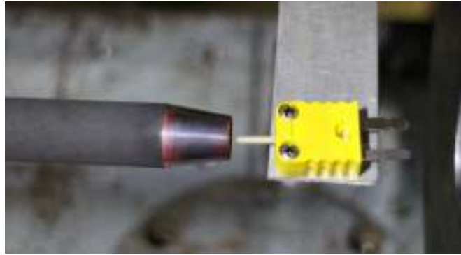
Figure 4.18: Photograph of test arrangement to determine the heating effect on the jet flow.
