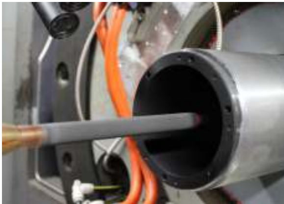
Figure 3.13: Mach 4 nozzle with internal surface painted black.
