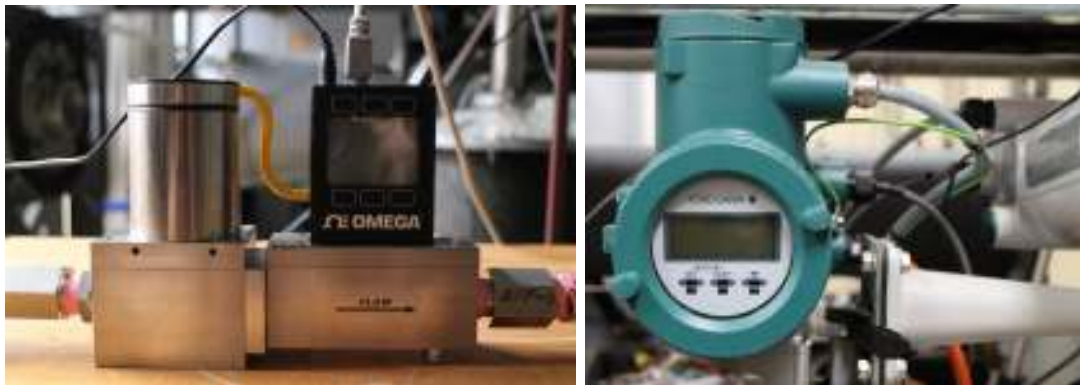
(a) OMEGA flow controller (a laminar flow device)
