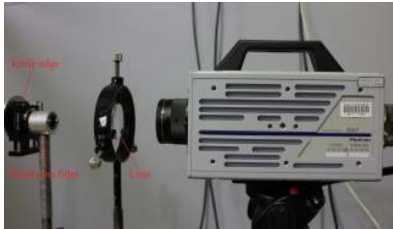
Figure 3.62: Photograph of high speed camera (Photron SA3).
