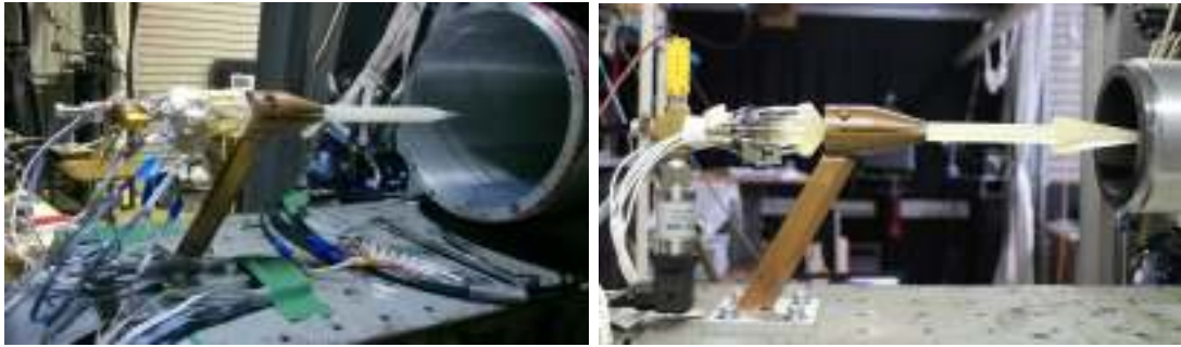
(a) Nose-cone installation with Mach 6 nozzle (b) Step-cone installation with Mach 4 nozzle
