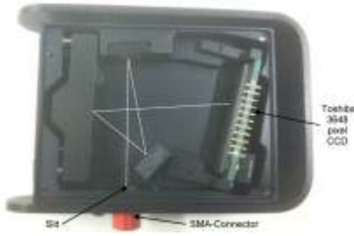
Figure 3.54: Top view of the opened CCS175 Spectrometer (Kraetzig, 2013).
