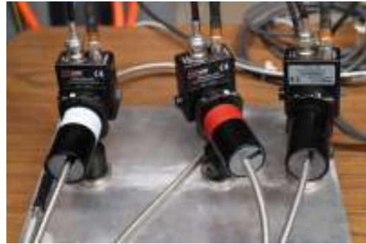
Figure 3.51: The set of Thorlabs amplified photodetectors used in the TCRP.
