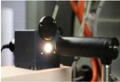
Figure 3.50: Integrating sphere used for calibration (on left) and an optical calibration tube (on right).
