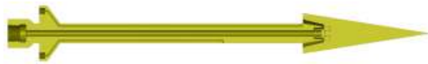
Figure 3.32: CAD view of the 3D printed step-cone model.
