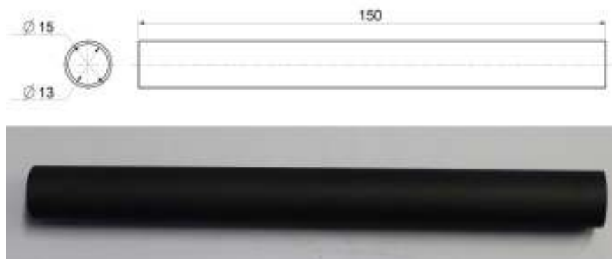
Figure 3.16: Dimensions and photograph of the type of graphite tubes.
