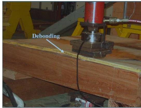
Figure 2.7 Debonding failure between sandwich core and skins (Islam & Aravinthan 2010)
