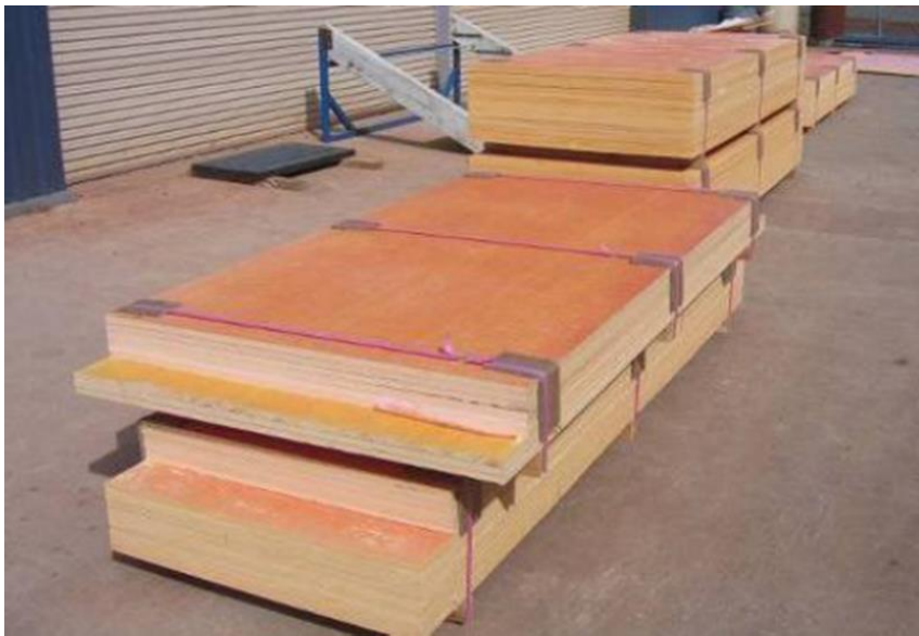
Figure 2.3 Novel GFRP panels (produced by LOC composites) ready to be transported to site (Aravinthan 2008)
