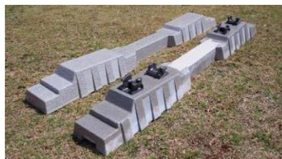
Figure 2.5 Sleeper made of polymer concrete and fibre composites (Manalo et al. 2010a)
