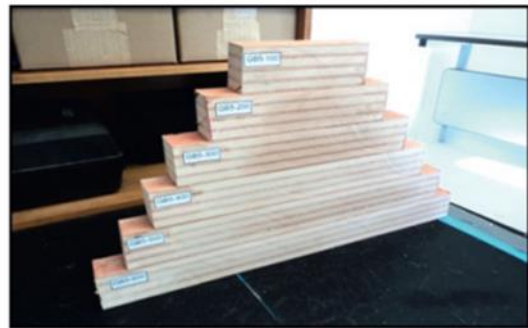
(b) Four layer glue laminated GFRP sandwich beams
