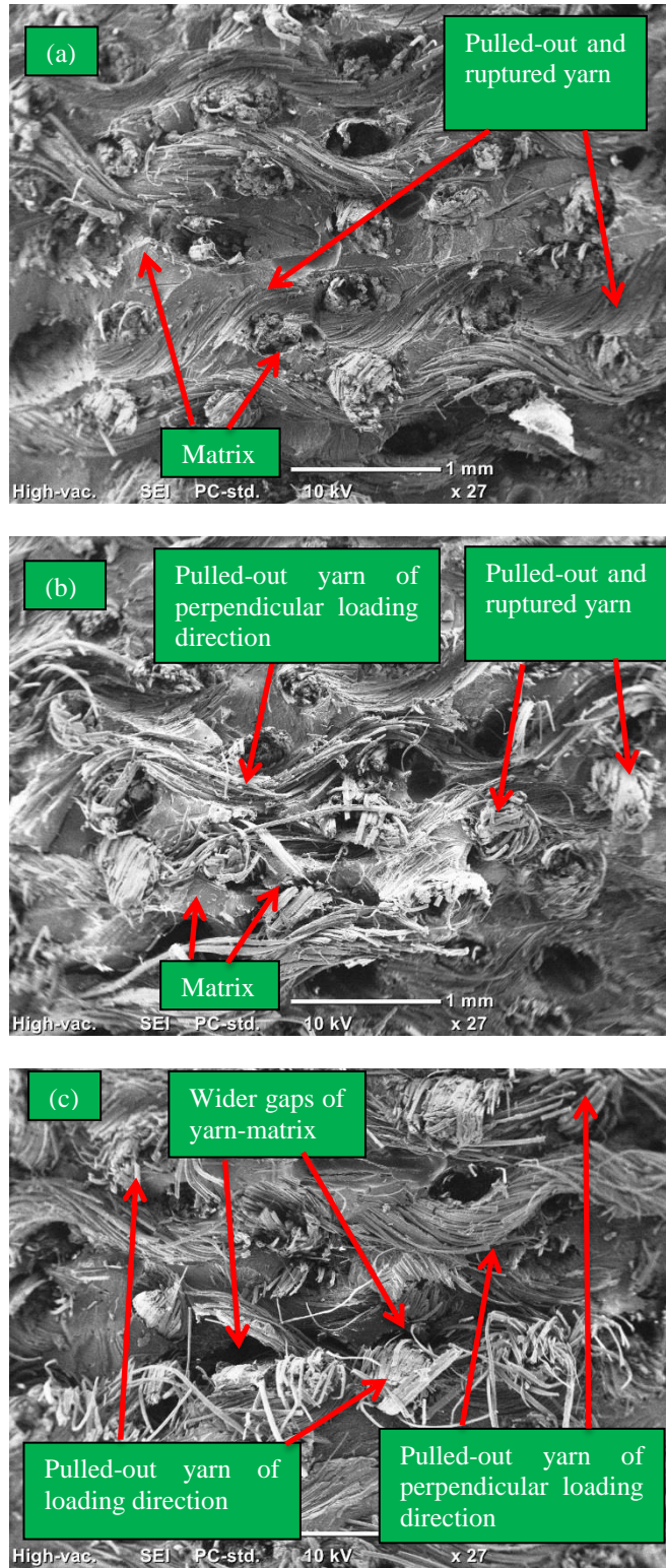
Figure 7.9 Scanning electron image of sample HVE-FR; (a) 0 hr, (b) 840 hr and (c) 2688 hr water immersion.
