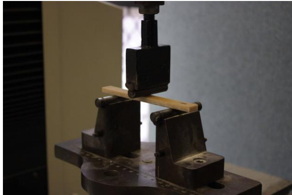
Figure 4.2 Flexural test setup with MTS Alliance RT/10 machine.
