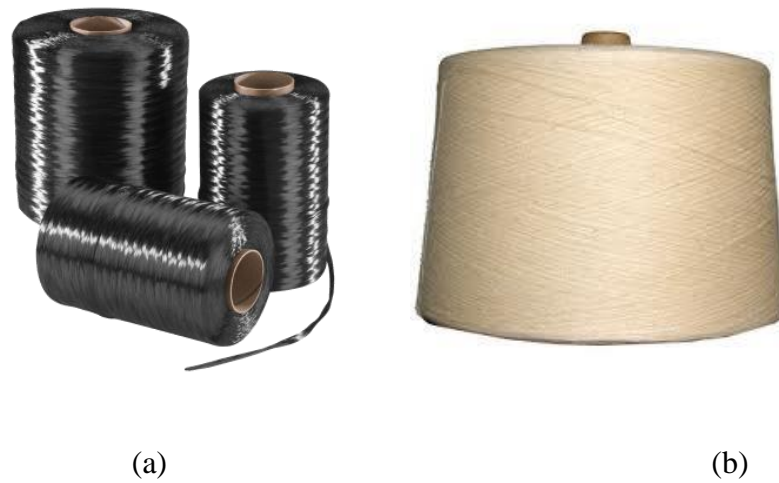
Figure 2.2 Example of yarn, (a) Carbon tows and (b) Cotton yarns [53].
