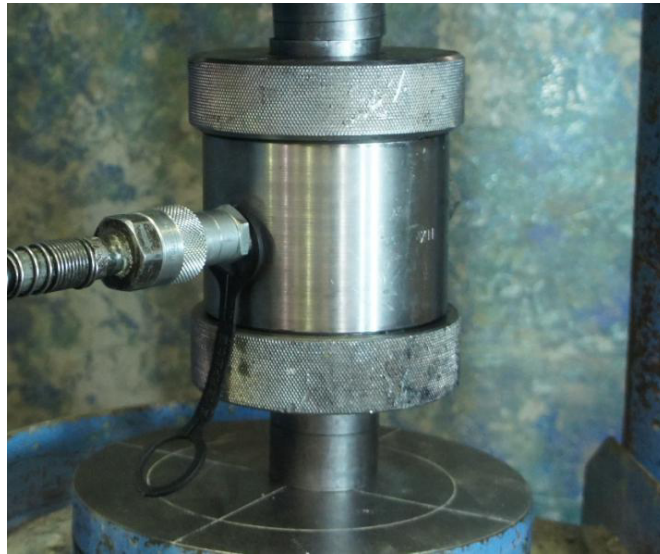
Fig. 6. Triaxial cell in testing arrangement.
