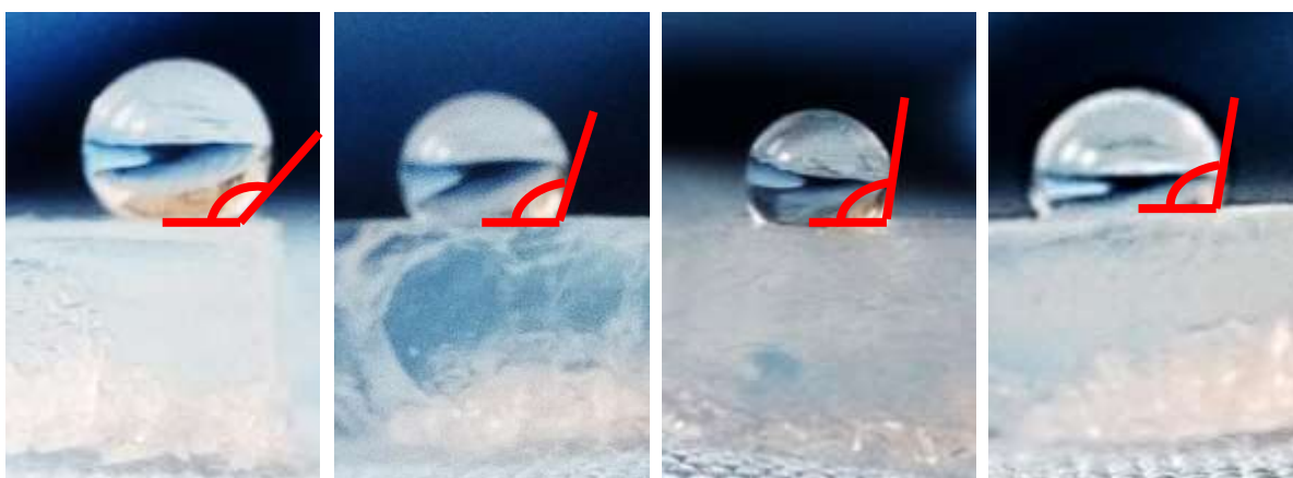
Figure. 3 3M water repellency solutions. (A) 100/0, (B) 90/10, (C) 80/20, (D) 70/30 water/alcohol drops on the aerogel surface
