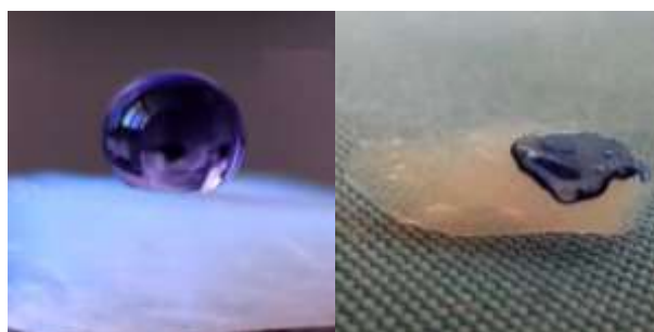
Figure. 4 (A) A (100%) water droplet, and (B) (60/40) water/Isopropan 2-ol drop on the synthesized aerogel surface.
