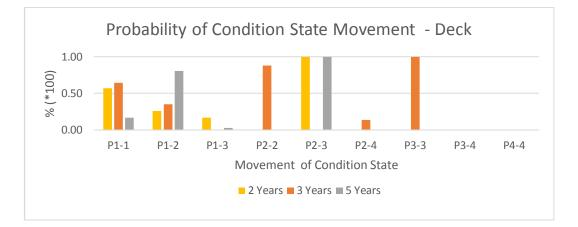
Figure 4.1 - Probability of Condition State Movement – Deck
