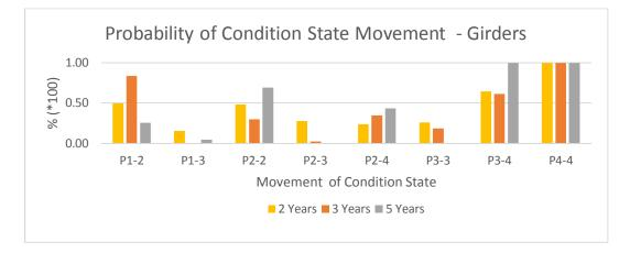
Figure 4.3 – Probability of Condition State Movement – Girders
