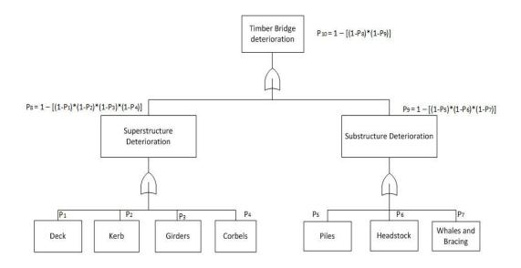
Figure 3.2 – Fault Tree Analysis model
