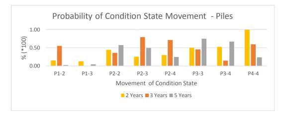
Figure 4.5 – Probability of Condition State Movement - Piles
