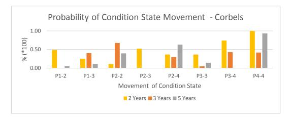
Figure 4.4 – Probability of Condition State Movement - Corbels
