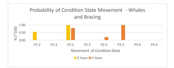
Figure 4.7 – Probability of Condition State Movement – Whales and Bracing
