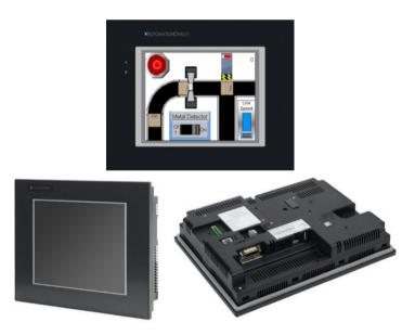
Figure 16: HMI C-more Touch Panels (Automation Direct 2016)
