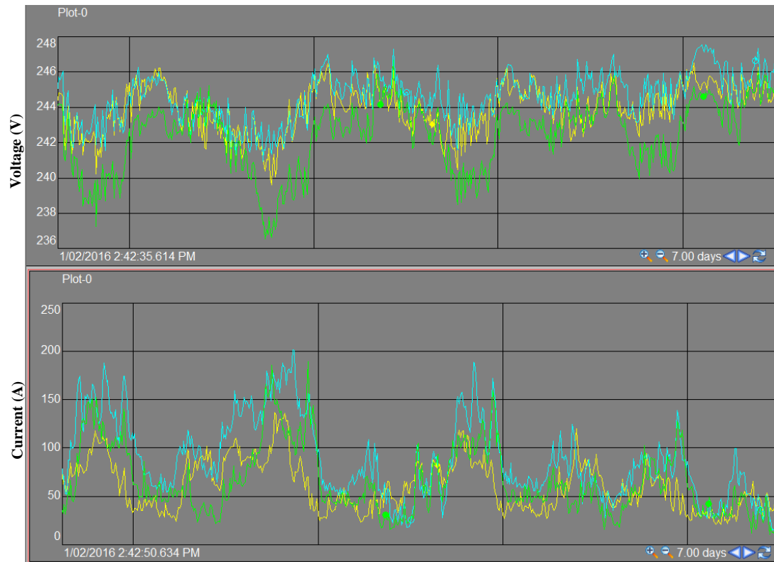
Figure 1.8 – Voltage and current measured at transformer at site 2 by Energex
