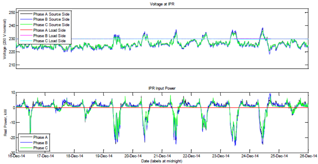
Figure 2. 10 – Measured Voltage at Source side and Load side of IPR and IPR Input Power by Leitermann, Olivia et al. 2015
