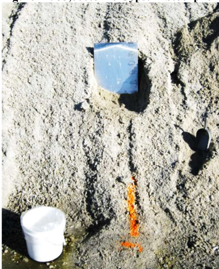
Figure 23: Gypsum Sampling using Stockpile Shield and sample scoop
