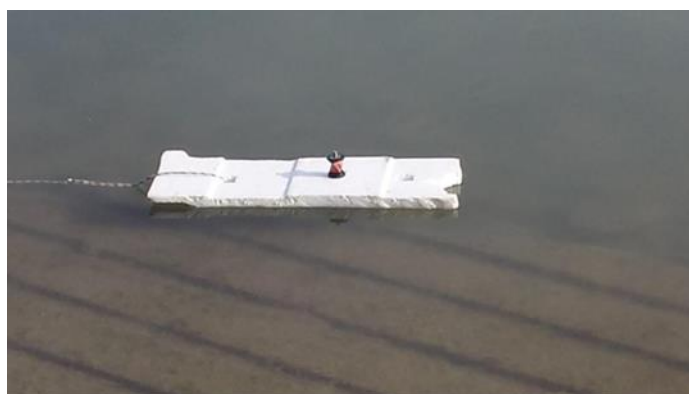
Pat's tide measuring device
