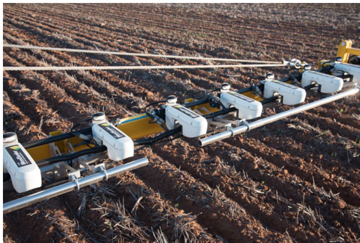
Figure 2.3: WeedSeeker Configuration on a common sprayer (Southern Precision2015)
