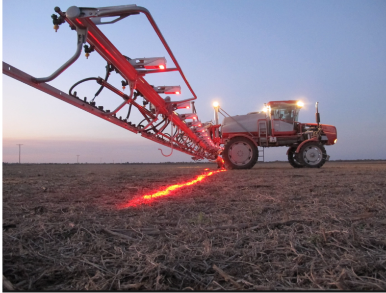
Figure 2.1: WEEDit configuration on a common sprayer (Romertron 2016)
