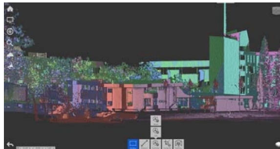
Figure 4.9: Point cloud colour based on scanning position
