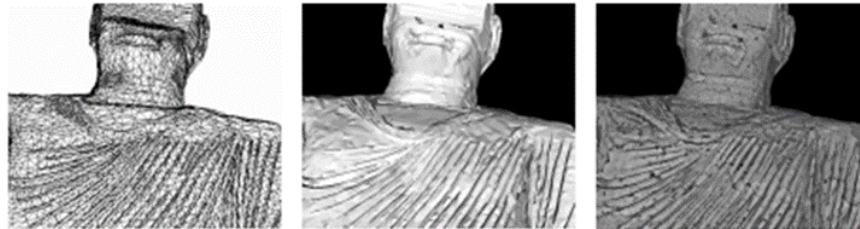
Figure 2.13: A closed view of a 3D model of the Bamiyan Buddha represented in wireframe, flat shade and texture mode (Gruen, Remondino & Zhang 2002)
