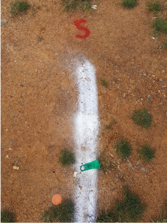
Figure 17. Photo at chainage 5 showing location detected on the surface
