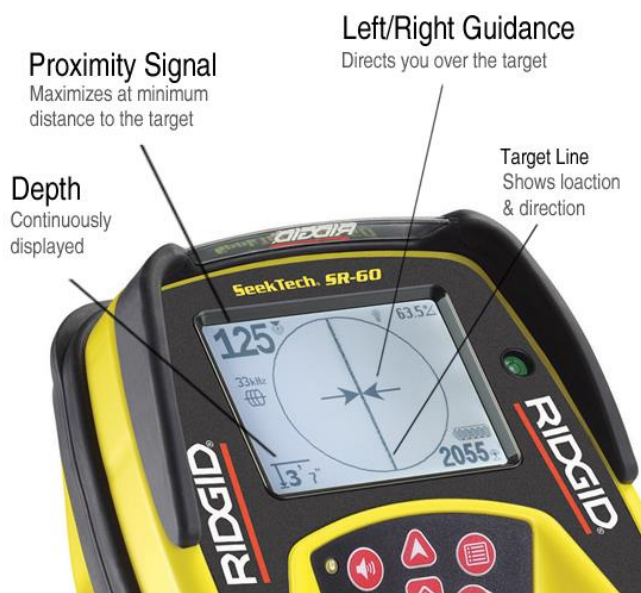
Figure 7. Typical screen of a modern receiver
