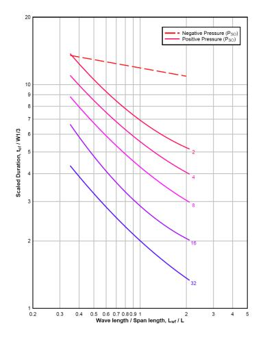
Figure 3-15. Scaled Duration of Equivalent Uniform Roof Pressures
