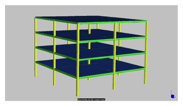
Figure 3-28. Reinforced Concrete Framed Building FE Structural Model
