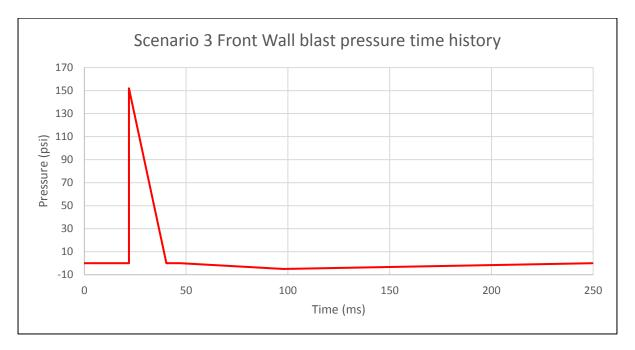
Figure 3-11. Scenario 3 Blast pressure time history at front wall
