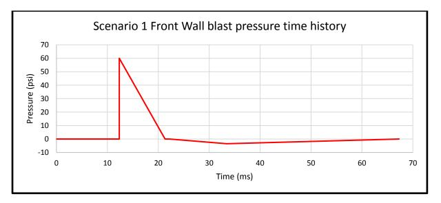
Figure 3-8. Scenario 1 Blast pressure time history at front wall
