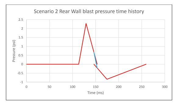
Figure 3-24. Scenario 2 Blast pressure time history of Rear Wall
