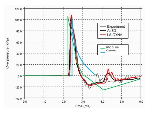
Figure 2-12. Comparison of Blast Pressure Time History Prediction Methods
