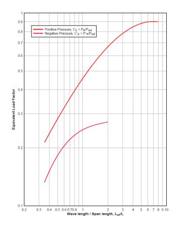
Figure 3-13. Peak Equivalent Uniform Roof Pressures
