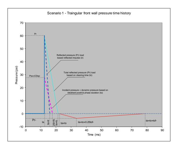
Figure 3-7. Blast pressure time history at front wall
