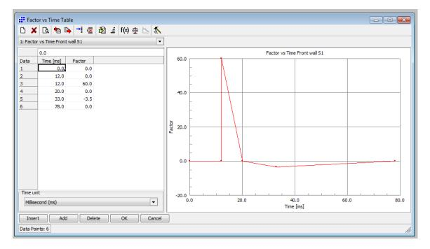
Figure 3-37. Factor vs Time Table for Blast Load Cases
