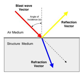
Figure 2-8. Refraction and reflection of blast waves interacting with two mediums (Source: adapted from USQ Study book MIN2001 Drilling and Blasting)
