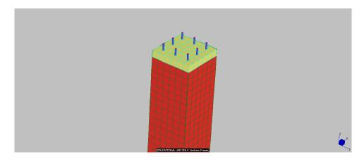
Figure 3-47. Reinforced Concrete Column with Wrapped in Steel Plate
