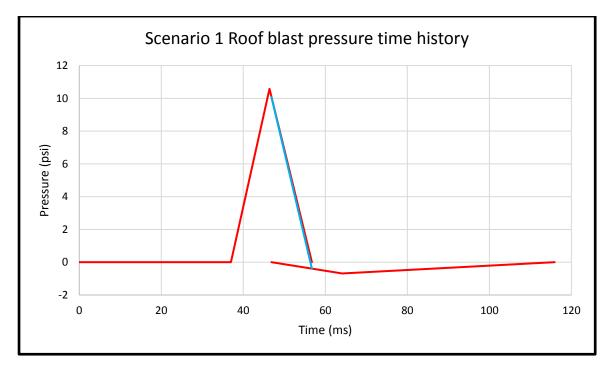
Figure 3-20. Scenario 1 Blast pressure time history for Roof
