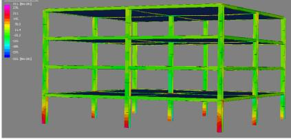
Time step 40ms end of front wall positive phase duration
