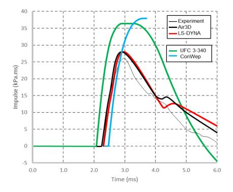
Figure 2-13. Comparison of Blast Impulse Time History Prediction Methods
