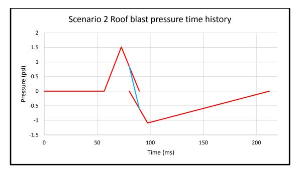
Figure 3-21. Scenario 2 Blast pressure time history for Roof
