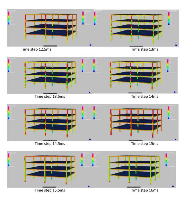
Scenario 1 concrete frame building displacements at floor levels contained below.
