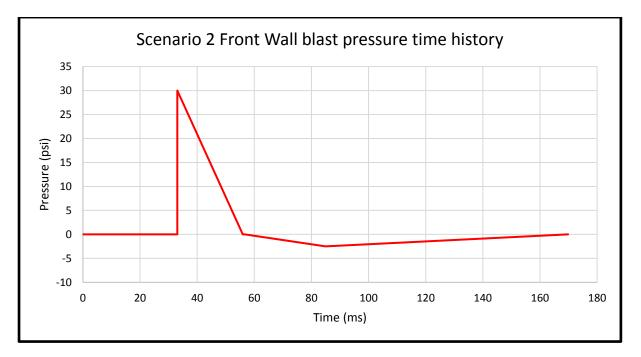
Figure 3-10. Scenario 2 Blast pressure time history at front wall
