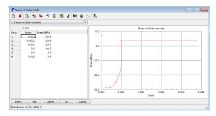
Figure 3-41. Concrete stress vs strain curve
