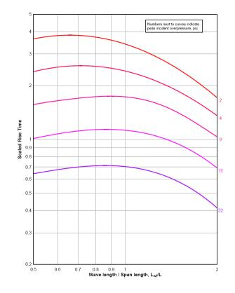
Figure 3-14. Scaled Rise Time of Equivalent Uniform Positive Roof Pressures
