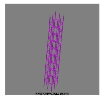
Figure 3-30. RC Column Reinforcement Detailing
