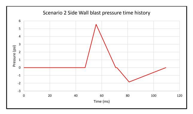
Figure 3-18. Scenario 2 Blast pressure time history at side wall
