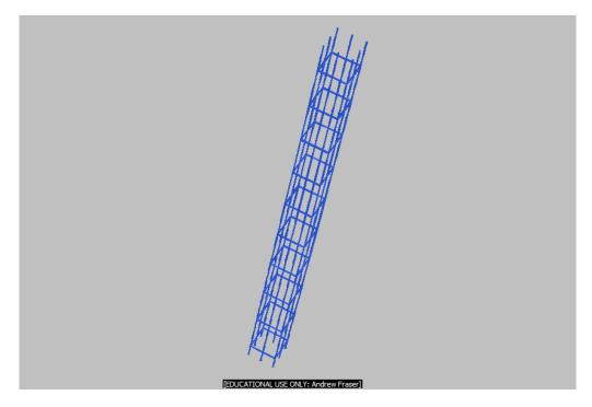
Figure 3-46. Reinforced Concrete Column Reinforcement Detailing
