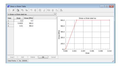
Figure 3-42. Steel stress vs strain curve
