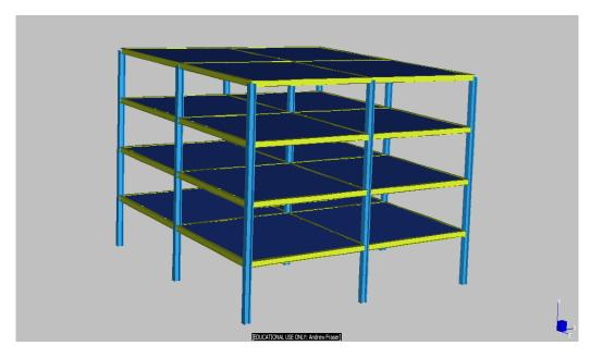
Figure 3-33. Steel Framed Building FE Structural Model
