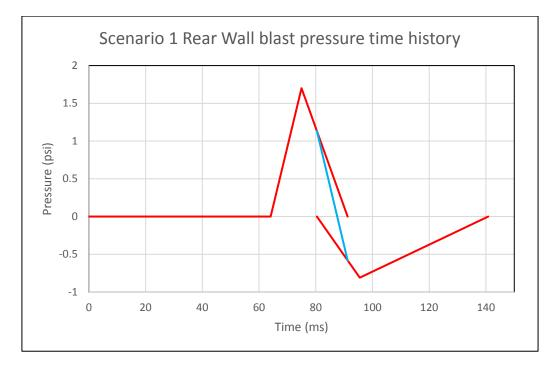
Figure 3-23. Scenario 1 Blast pressure time history of Rear Wall
