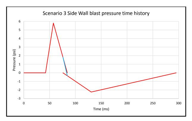
Figure 3-19. Scenario 3 Blast pressure time history at side wall
