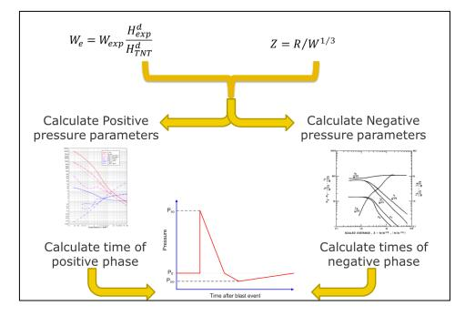
Figure 2-10. UFC-340-02 Procedure for determining blast pressure time history curves
