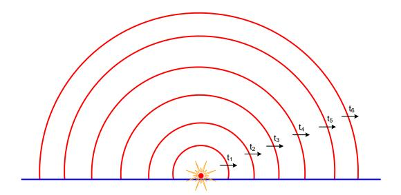
Figure 2-1. Surface blast
