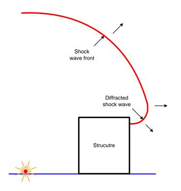
Figure 2-7. Blast wave diffraction
