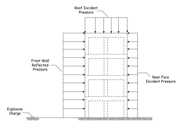
Figure 3-26. Elevation Diagram of Typical Structural Model Peak Blast Loading Interaction
