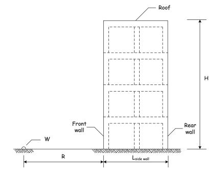
Figure 3-1. Model Structure Subjected to Blast Action (elevation)
