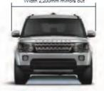
**Obstacle Clearance** Off-road height up to 310mm Standard ride height up to 185mm
