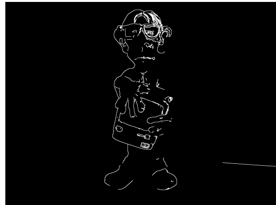
Figure 1.14: Canny edge detection applied to the figurine and edges dilated.
