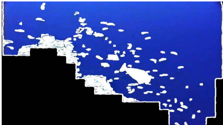
Figure 2.4: Blobs detected after edge detection, coral blackening and blob filling.
