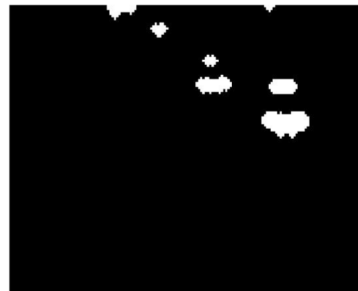
Figure 2.12: Background subtraction and blob analysis performed to identify white cars.
