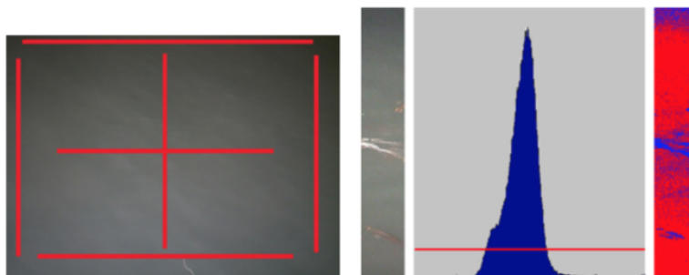
Figure 2.6: Frame divided into different areas and histogram bin thresholding applied.
