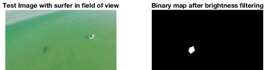
Figure 5.6: Morphology applied to frame with a surfer in the field of view.
