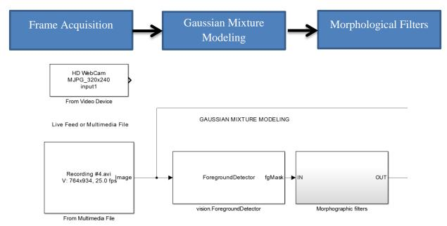
Figure 14 - GMM and Morphological Filter Simulink Model
