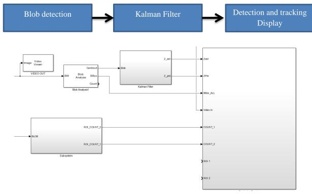
Figure 16 - Blob analysis, Kalman Filter and Display Simulink Model
