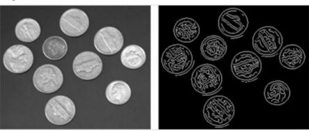
Figure 3 - Canny Method
