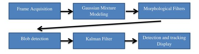
**Frame Acquisition** – Video input separated into frame by frame in order to process changes in pixels.
