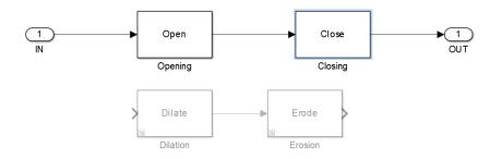
Figure 15 - Morphological filters subsystem
