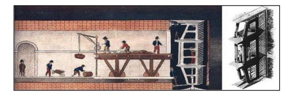
Figure 2.2: Brunel's shield, a diagram showing a longitudinal section and one of the twelve frames (Guglielmetti et al. 2007).
