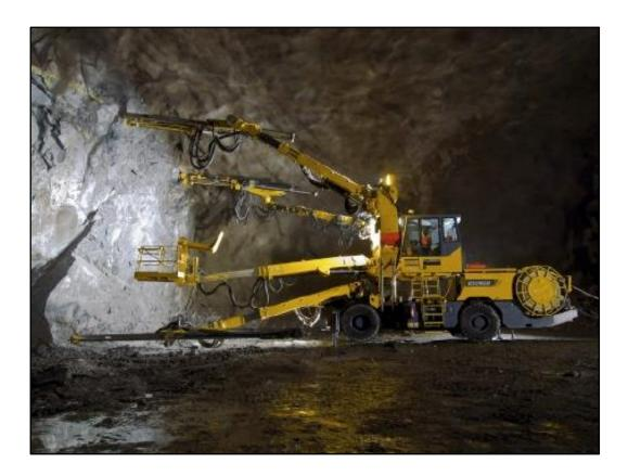
Figure 2.5: Typical face drilling rig used in drill and blast tunnelling (Atlas Copco 2014).
