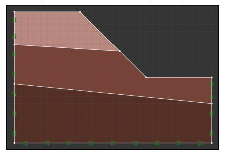
Figure 3.9: Material types assigned to layers (Optum Computational Engineering 2016).
