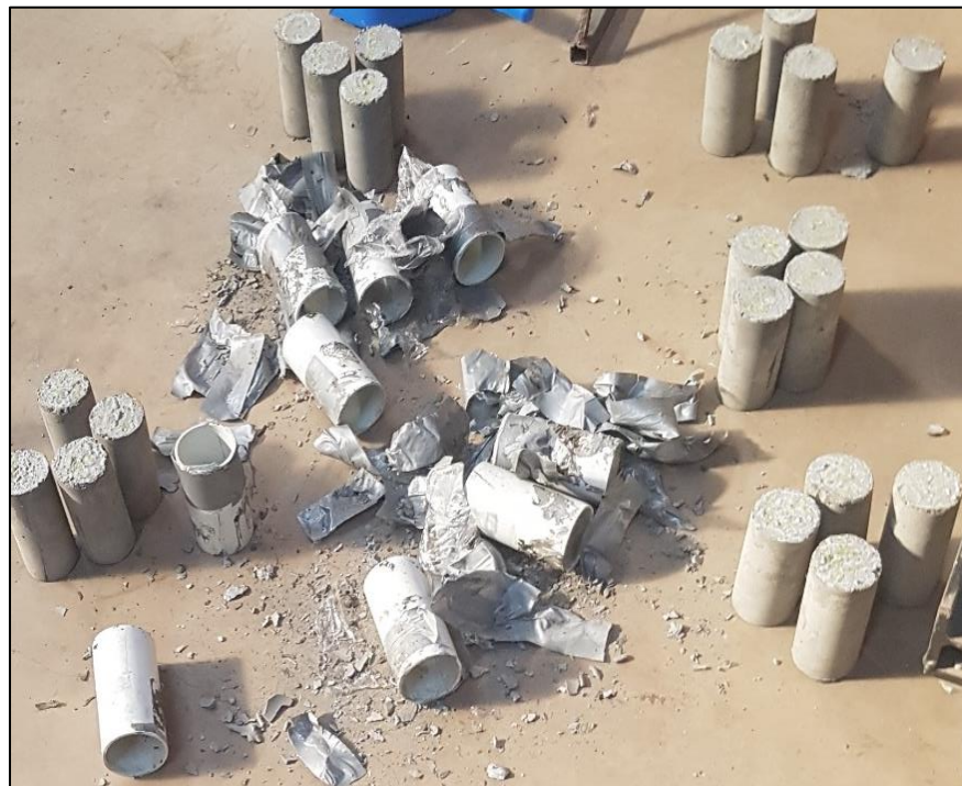
Figure 3. 8 Prepared samples of cements with different ratio of waste ceramic aggregates
