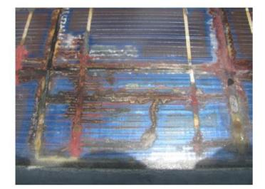
Figure 2.29 - 85/85 cell degradation after 3500 hours in harsh conditions (Wohlgemuth et.al, 2010).
