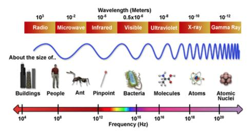
Figure 2.2 - Electromagnetic spectrum (Science UK, 2016).
