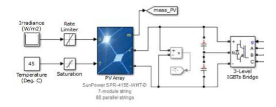
Figure 2.32 - PV array example showing irradiance and temperature control (Mathworks, 2016).
