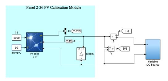
Figure 3.11 - Panel 2-36 calibration model.
