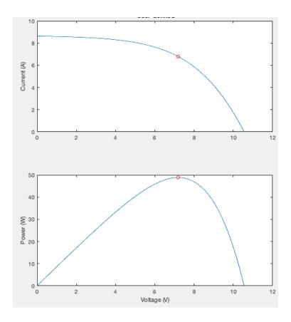
Figure 3.10 - Single panel @1000W/m<sup>2</sup> and 100% panel  $90^{\circ}$ C – 48.80W.
