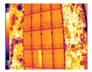
Figure 2.7 - Failed bypass diode, Thermography 1/3 of panel failed (Tsanakas 2016).
