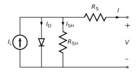
Figure 2.16 - Circuit model, using a series and parallel resistance and a single diode (Eitner *et.al* 2010).
