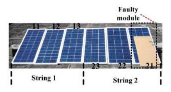
Figure 2.24 - Simulation of faulty panel using a shade shield (Hu et.al, 2013).
