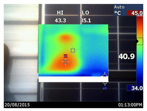
Figure 4.9 - 1<sup>st</sup> major cell failure detection 7.3°C hot spot, approximately 40% cell coverage.
