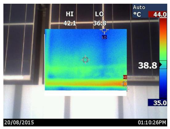
Figure 4.6 - Panel temperature lowered from 41.3 - 36.8°C after cleaning.
