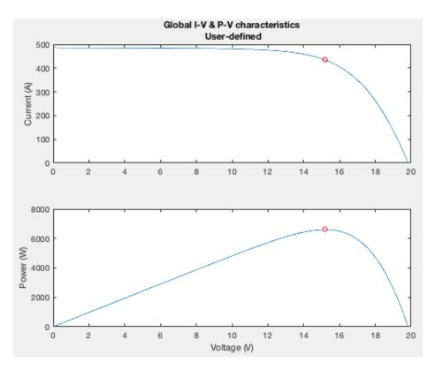
Figure 5.2 - Total output of 36 x dirty panels @ 42°C.
