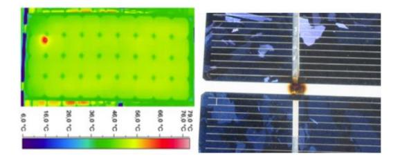
Figure 2.5 - Solder/ribbon degradation small hotspot (left) visual degradation (right) (Tsanakas 2016).
