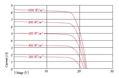
Figure 3.6 - Kyocera KD135GH-2PU I-V data sheet characteristics @25°C at various irradiance levels, (Kyocera, 2010).
