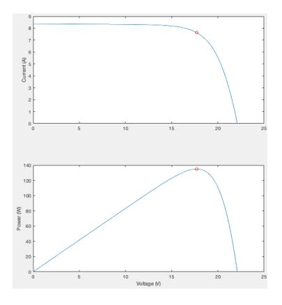
Figure 3.1 - Single panel @1,000W/m<sup>2</sup> at  $25^{\circ}C - 135.04W$ .
