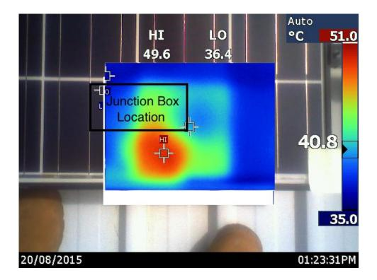
Figure 4.19 - Junction box indication, to confirm heating was not coming from junction box area.
