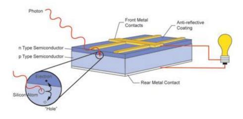
Figure 1.2 - PV effect basic diagram (Viridian, 2016).
