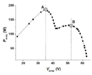
Figure 2.26 - P–V plot with the module covered (Hu et.al, 2013).
