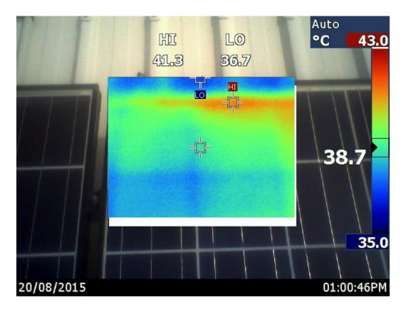
Figure 4.5 - Effects of ingress and dirt on array.
