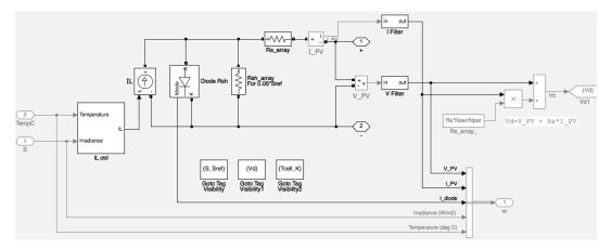
Figure 2.33 - Detailed Simscape PV array logic (Mathworks, 2016).
