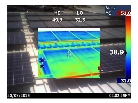
Figure 4.17 - Healthy panels from a distance, no visual signs of hot spots.
