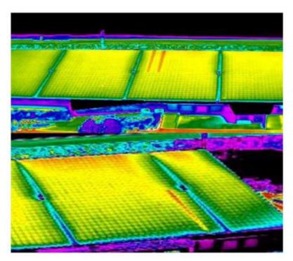
Figure 2.22 - Multiple panels with increased temperatures in this large PV system (Denio, 2011).
