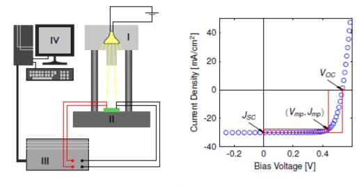
(a) J-V set-up (b) J-V curve example
