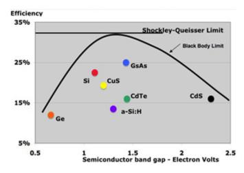
Figure 2.1 - Panel type efficiencies and Skockley-Queisser limit for a single junction cell (Solar Central, 2016).
