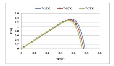
Figure 2.18 - Temperature effects on PV output (Salmi, 2012).
