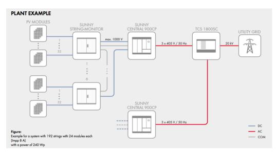
Figure 2.30 - Sunny string-monitor plant example diagram (SMA, 2016)
