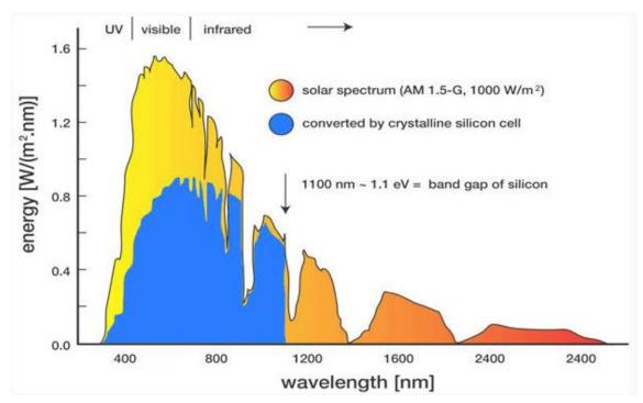
Figure 2.3 - Typical crystalline silicon cell wavelength conversion spectrum (Viridian, 2016).
