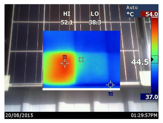
Figure 4.13 -  $5^{\text{th}}$  detection  $16^{\circ}\mathrm{C}$  hot spot approximately 95% cell coverage.
