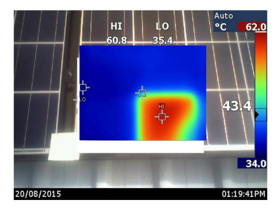
Figure 4.11 -  $3^{rd}$  detection – 24.8°C max hot spot 90% cell coverage.
