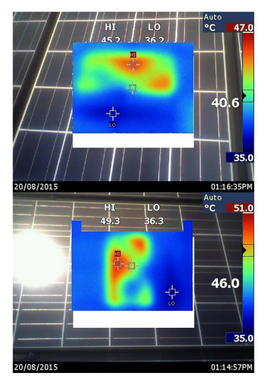
Figure 4.10 - Two images of the  $2^{nd}$  detection dual cell failures – 13.3°C max hot spot, approximately 50% cell coverage.
