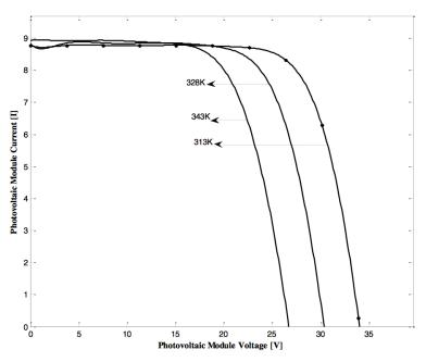
Figure 2.19 - Temperature effects on I-V curve (Savitha, 2014).
