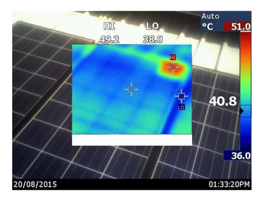
Figure 4.15 - Same 6<sup>th</sup> detection from distance hot spot stands out.
