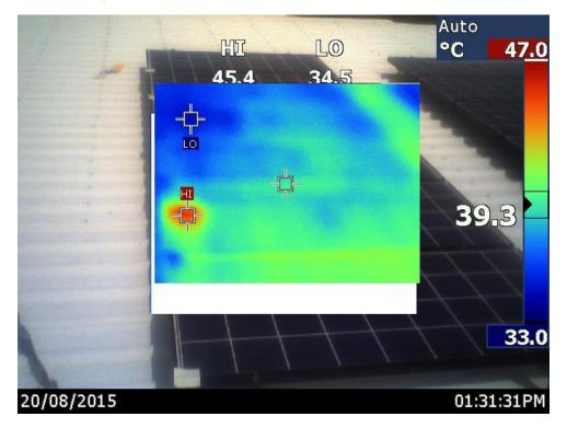
Figure 4.16 - 4<sup>th</sup> detection from distance hot spot stands out.
