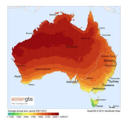
Figure 2.13 - Australia average global horizontal irradiation – (SolarGIS, 2013).
