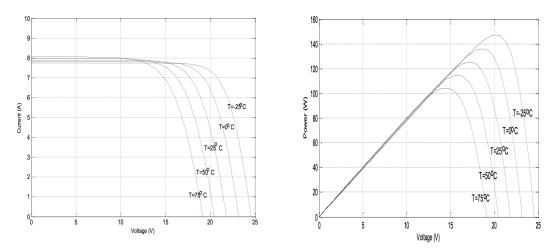
Figure 2.17 - (Left) I-V plots at set temperatures and allocated irradiance (Right) P-V plots Module's P-V plots at set temperatures and allocated irradiance (Krismadinata *et.al*, 2012).
