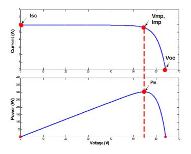
Figure 2.31 – P-I and P-V curve showing maximum power point relationship (Mathworks, 2016). Mathworks (2016) defines characteristic equation for the diode I-V for a single array as
