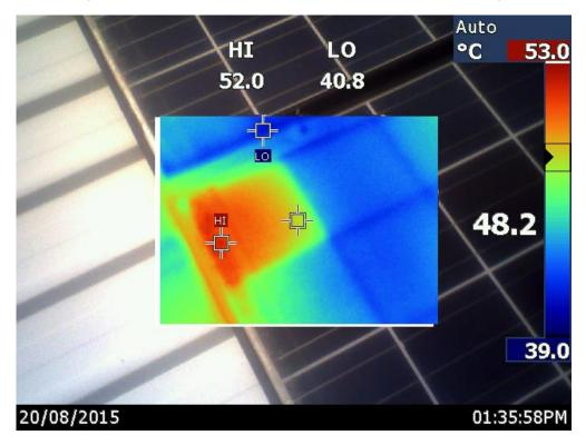
Figure 4.14 - 6<sup>th</sup> detection - 16°C hot spot approximately 95% cell coverage.
