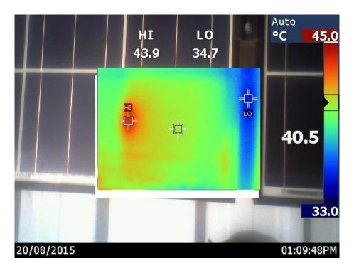
Figure 4.8 - Early cell failure signs 8°C hot spot approximately, less than 10% cell coverage.
