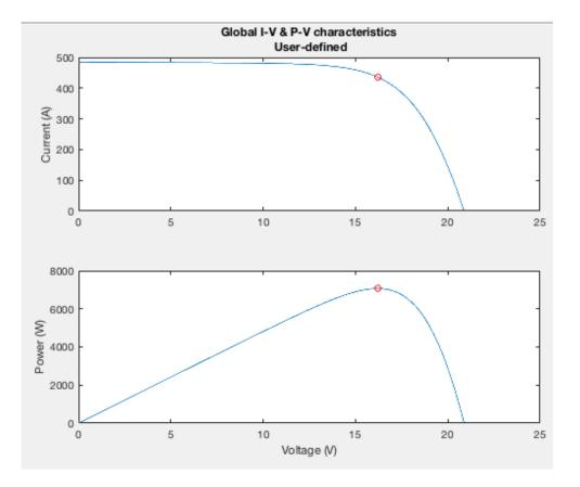
Figure 5.1 - Total output curves at  $61^{\circ}C$  hottest single cell model.
