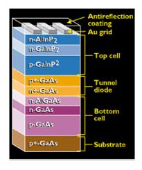
Figure 1.5 - Multi-junction stack example (NASA Science, 2016).
