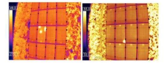
Figure 2.6 - Single cell thermograph hot spot (left) multiple cells failed shown in thermograph hot spot (right) (Tsanakas 2016).
