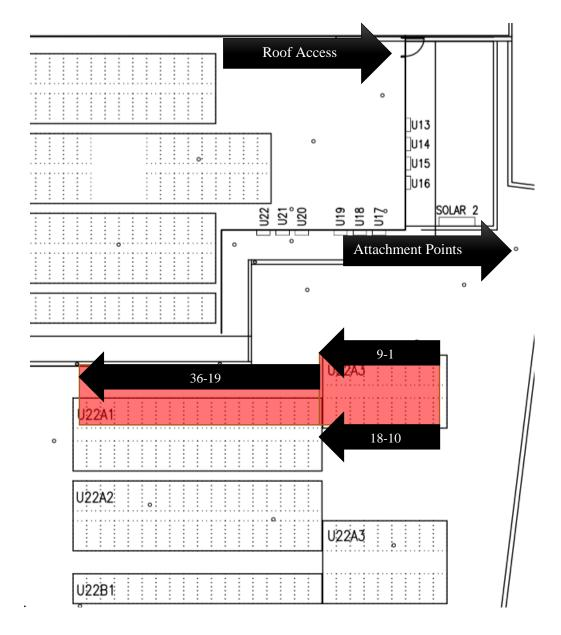
Figure 4.1 - Zoom of layout (Red) indicating the 36 panels scanned, access and attachment points (Appendix B full size).
