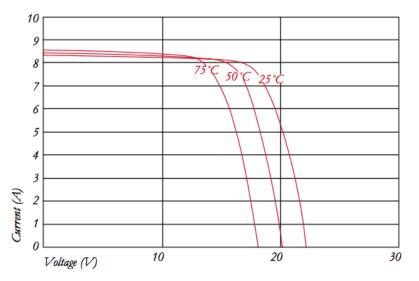
Figure 3.8 - Kyocera KD135GH-2PU module I-V data sheet characteristics @1000W/m<sup>2</sup> at various cell temperatures (Kyocera, 2010).
