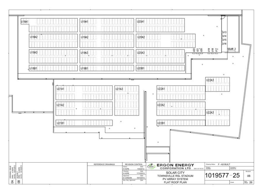
Figure 0.5 - Panel and invertor layout Townsville RSL Stadium flat roof plan.
