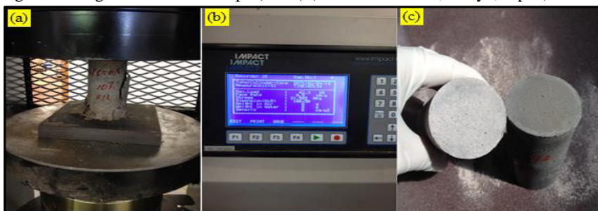
Figure 2: Compressive strength machine
