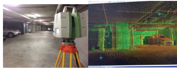
Figure 1 – Terrestrial Laser Scanning and resulting Point Cloud
