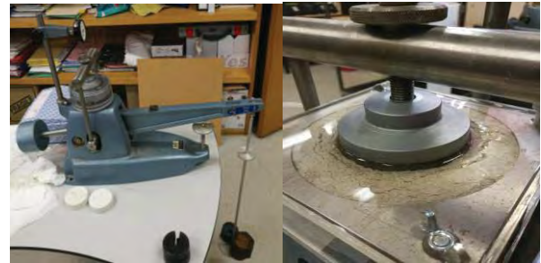
Figure 1 (left) – Oedometer with standard cell loaded
