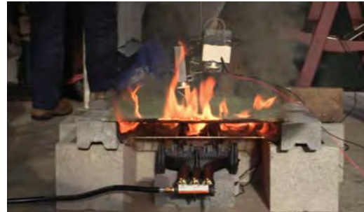
Figure 1 – CFRP Air-Coupled Ultrasonic Test Under Fire
