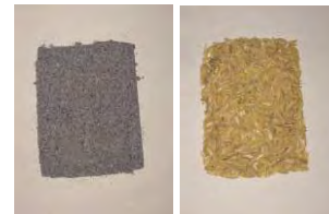
Figure 1 – Comparison of burnt & unburnt RHA
