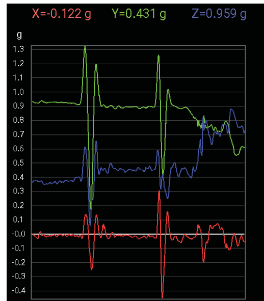
Figure 1 – G Force in the test vehicle driving over "Type 2" speed hump.
