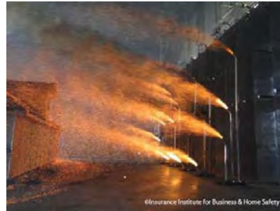
Figure 1 - Simulated Firebrand Attack
