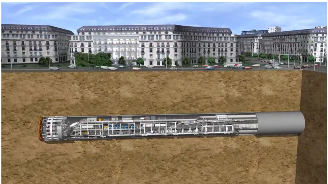
Figure 2-4 Cutaway depiction of a TBM operating underneath an urban area (courtesy of Herrenknecht )
