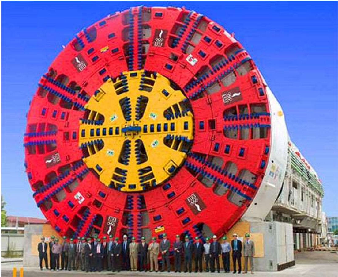
Figure 2-3 Photograph of TBM used in Madrid metro construction (courtesy of Herrenknecht )
