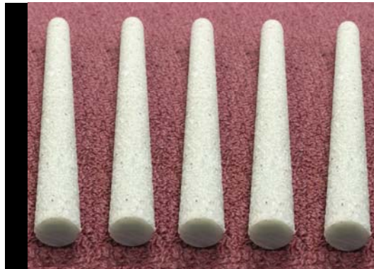
Fig. 1. 15.9 mm GFRP bars.
