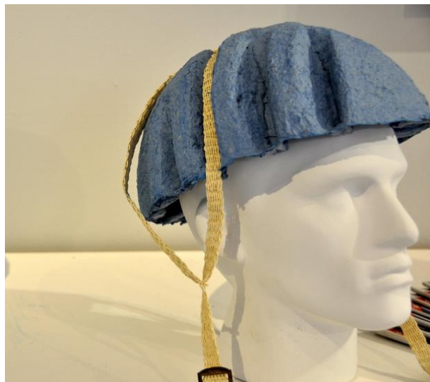
Figure 4.2 Paper Pulp Helmet Design
