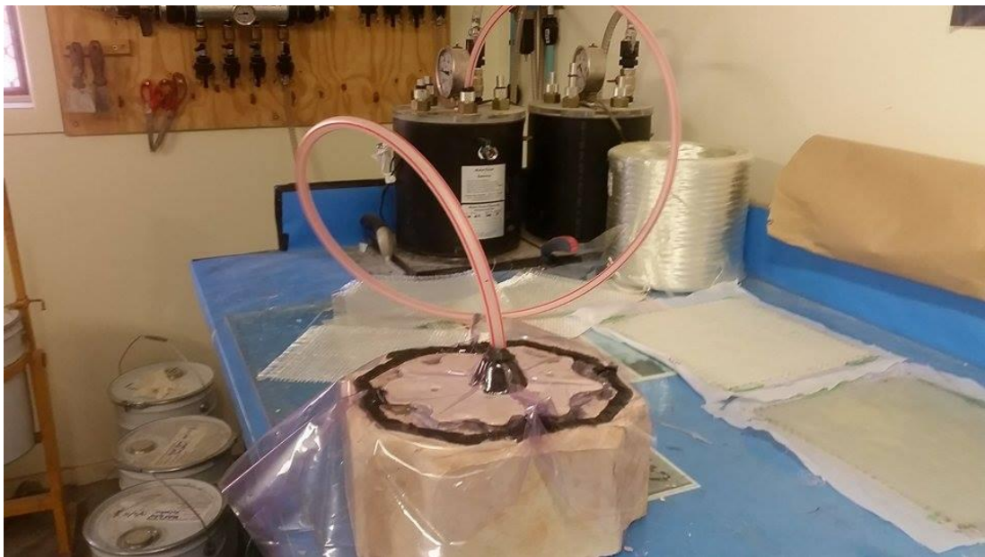
Figure 6.3, Vacuum compression technique of manufacturing helmets
