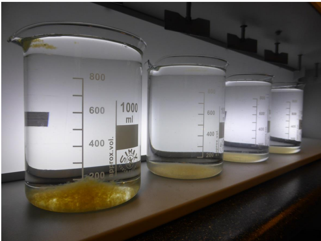
Figure 6-1 Water samples settling after the jar test with the selected optimum coagulant doses. From left: Japanese Gardens, Cooby Dam, Mt Kynoch raw water mixture, Perseverance and Cressbrook Dams
