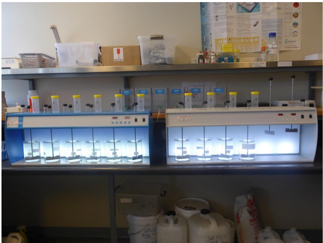
Figure 3-2 Jar testing experimental set-up
