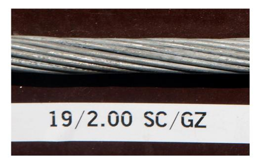
Figure 19: A close up photograph showing the typical surface characteristics of the actual galvanised steel conductors tested.
