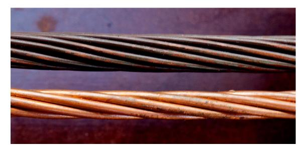
Figure 20: A close up photograph showing the different surface characteristics of the actual copper conductors tested.
