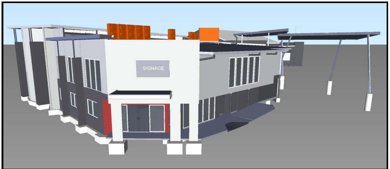
Figure 5.11 - 3D BIM Model (Building Approval Stage)
