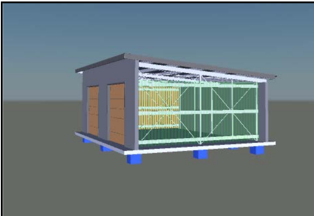
Figure 4.18 - Navisworks Manage Simulation – “wall complete and cladding under construction”
