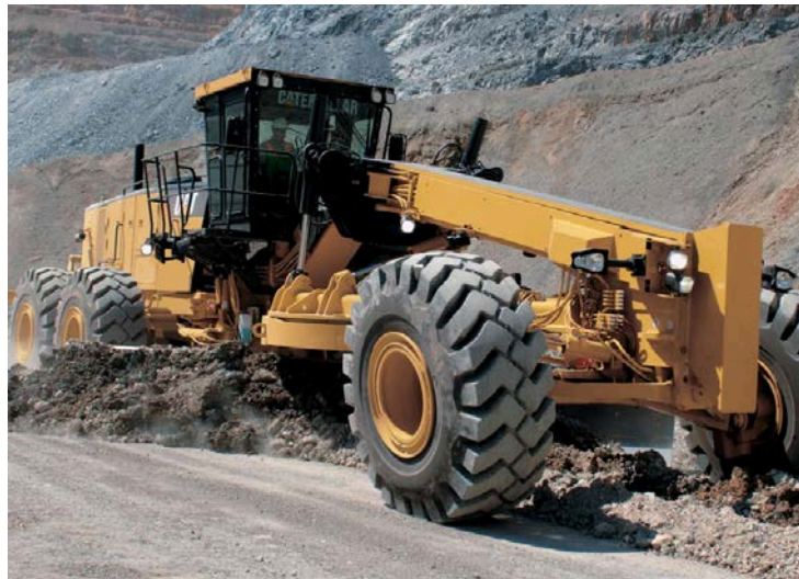
Figure 2: Grader conducting road maintenance (Caterpillar 2015)
