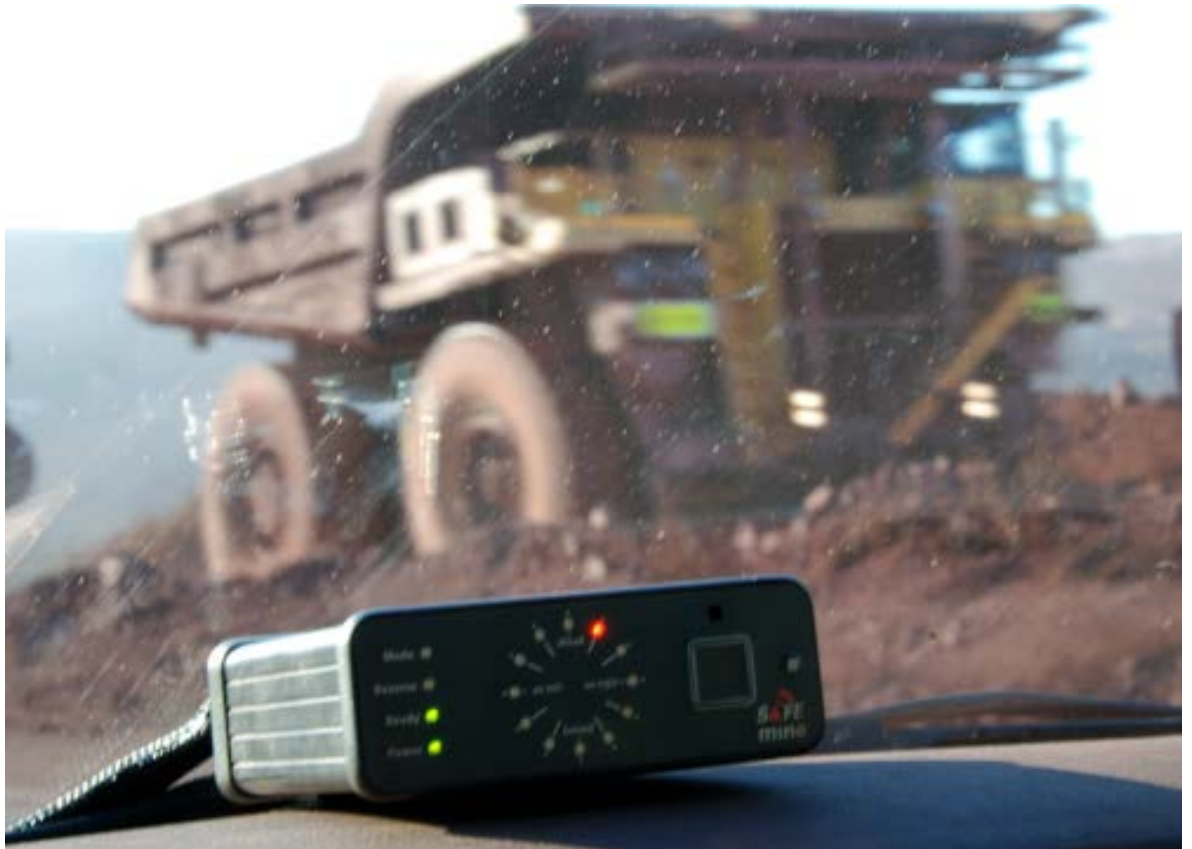
Figure 10: SAFEmine user interface shown in in vehicle cabin ( Our Products - SAFEmine CAS n.d.)
