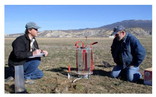
Figure 3–7: A Cornell Sprinkler Infiltrometer in use (Molacek et al. date unknown).
