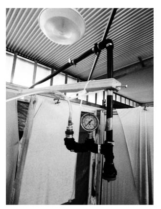
Figure 3–5: Sprinkler head set-up, with the pressure line to primary pressure gauge and the secondary pressure gauge shown.
