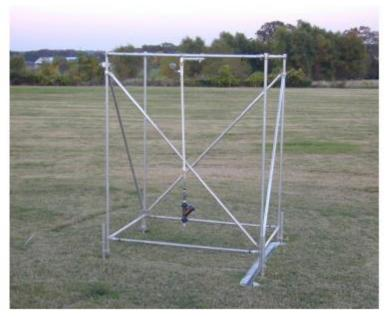
Figure 2–6: A portable rainfall simulator using a single pressurised nozzle. The plot area is 1.5m x 2.0m (Humphrey et al. 2002, Fig.1, p.201).
