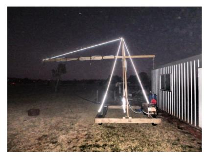
Figure 4–8: Photo of the rig before sunrise. Note the reflective ropes used to stabilise the structure and reduce sagging of the horizontal bar.
