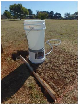
Figure 3–8: The 'bucket infiltrometer' used as a reserve sprinkler infiltrometer,.
