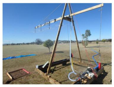
Figure 4–7: Photo of the mobile rig with sprinklers running. Note the flowmeter and pressure gauge at the bottom right.
