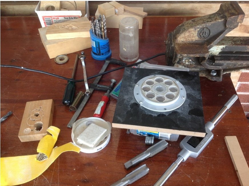
Figure C.7: Rotor magnets holes are being finalised to allow extra space for the adhesive.
