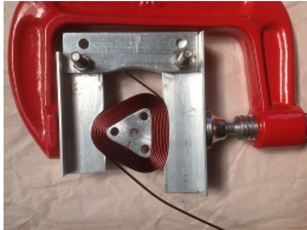
Figure 4.14: A wound coil with 8 turns.
