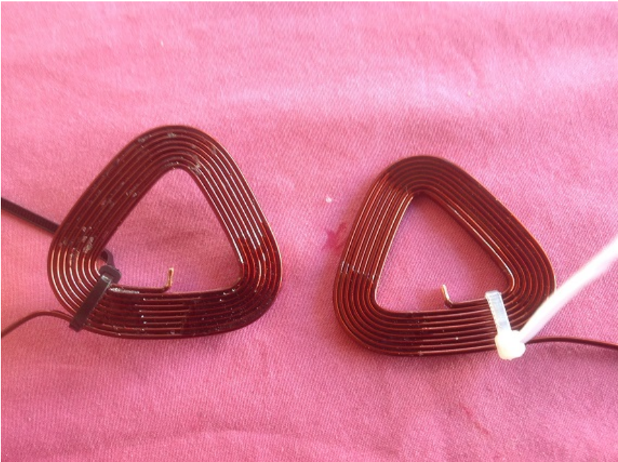
Figure C.16: Two single layer coils are correctly oriented for joining.
