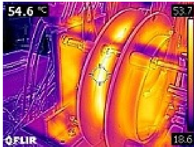
Figure 5.16: Stator temperature output after 20 minutes at 11A output current.
