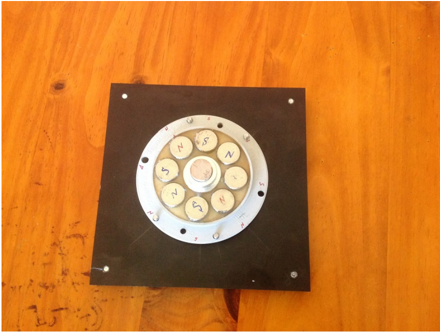
Figure C.10: Rotor magnets are set with Araldite Selleys Epoxy Adhesive. There is a fillet of Araldite between the surfaces of polyester resin (core) and the magnets to provide an extra bond. The magnets' pole surfaces are free of any epoxy.
