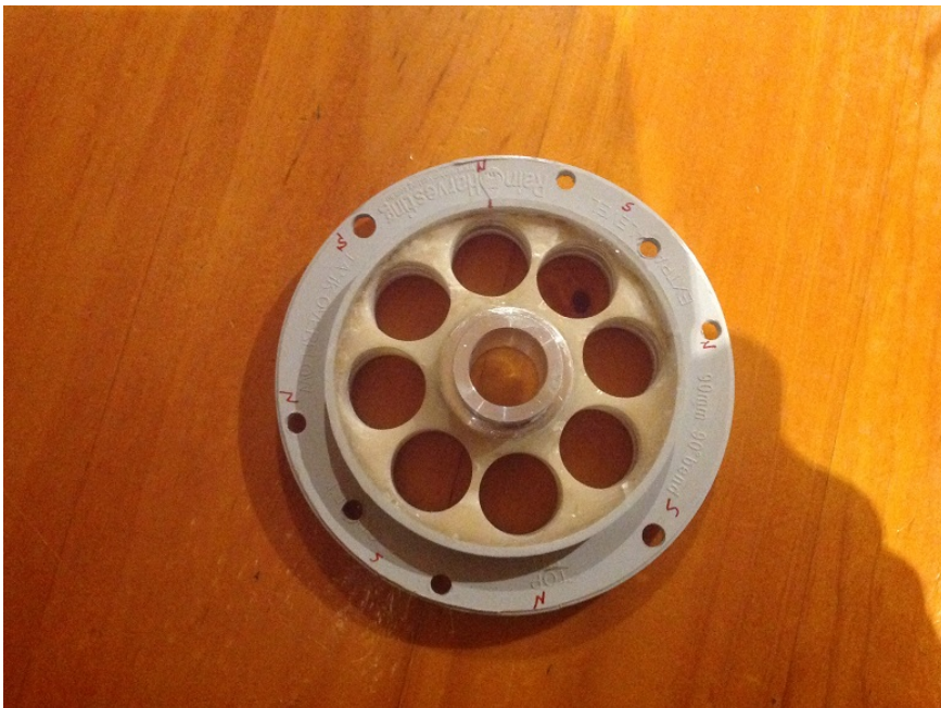
Figure C.9: Rotor supporting structure is ready magnets (top side). There are imperfections in the surface finish. The magnets' placements are marked N, S to accommodate magnets' magnetic poles.
