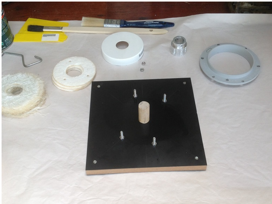
Figure C.1: Rotor setup parts from left to right: pre-cut Fibreglass Chopped Strand Mat (CSM) 300gm, pre-cut Fibrecore 3mm Fibreglass, press plate, Rotor Bushings, former flange. The CSM adds structural strength to the core, while the Fibrecore gives extra body to the core.
