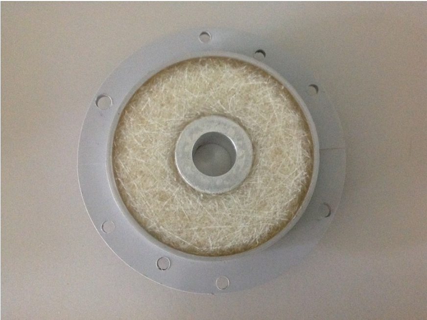
Figure C.4: Rotor former set with polyester resin (bottom side). CSM is clearly visible on the photograph.
