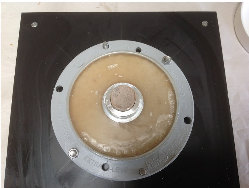
Figure C.3: Rotor former set with the polyester resin (Top side).
