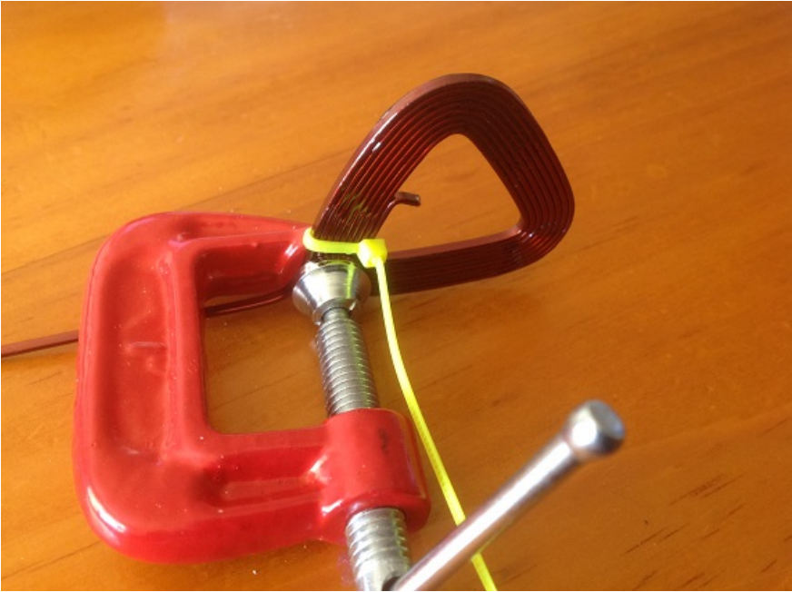
Figure C.15: Araldite is applied to the sides of a single layer coil.
