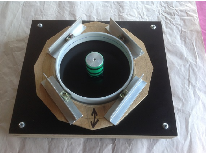
Figure C.18: The stator mould.
