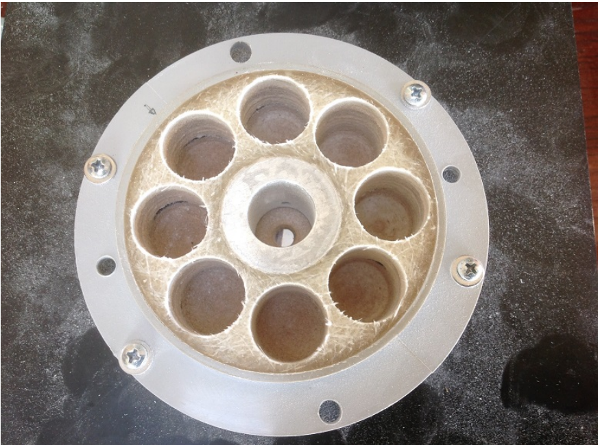
Figure C.6: Rotor magnets holes are partially drilled.
