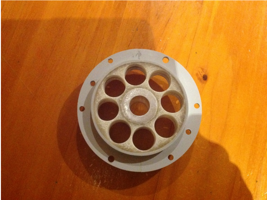
Figure C.8: Rotor supporting structure is ready for magnets (bottom side).
