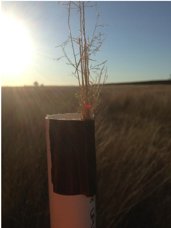
Reflectorless Laser Beam on Light Vegetation
