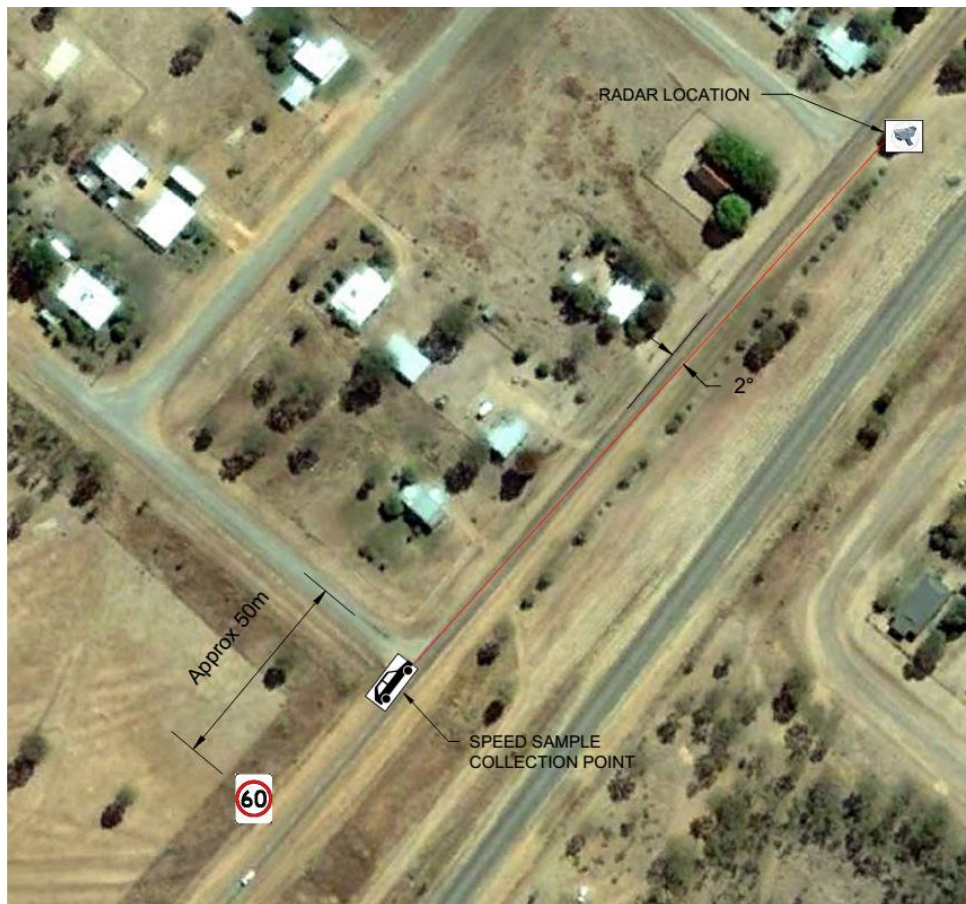
Figure 6.24: Pentland west approach – speed sample survey layout
