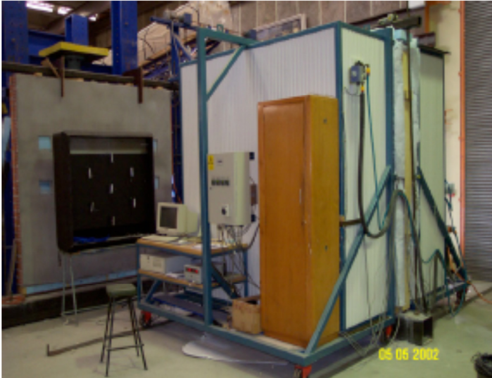
Figure C.2 – A guarded hot box apparatus in use
