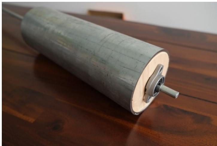
Figure 4.7: Mock-up of the test roller
