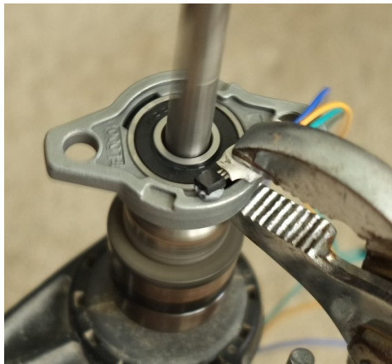
Figure 6.2: Actual location of temperature sensor
