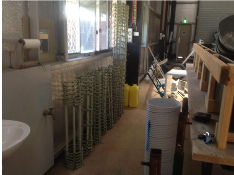
Figure 3.6: The constructed reinforcement cages.
