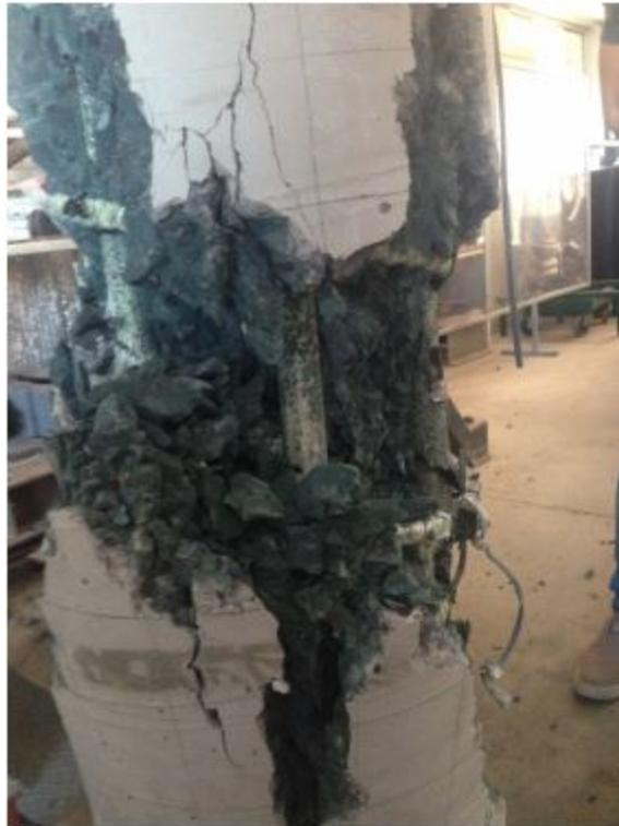
Figure 4.26: The core crushing of specimen S1-100.
