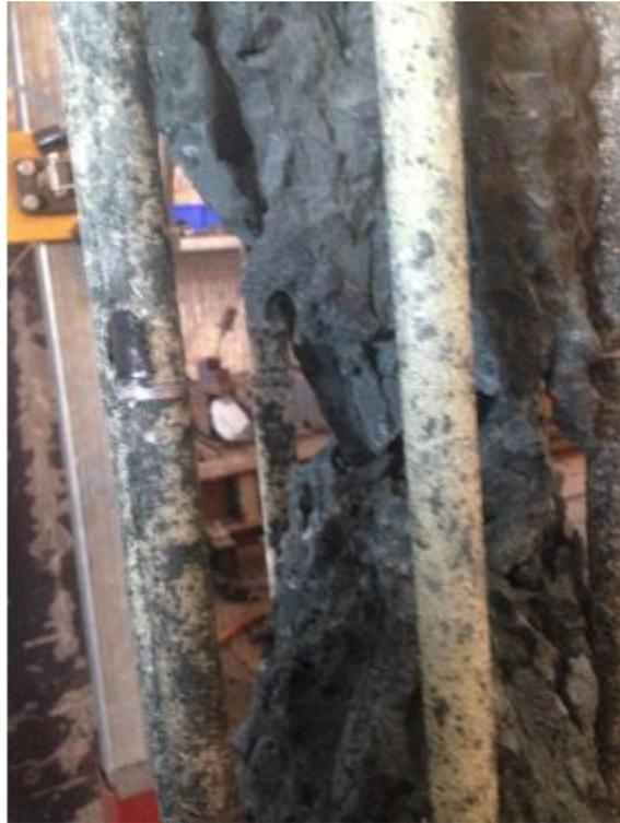
Figure 4.2: Core crushing failure of specimen C1-0.
