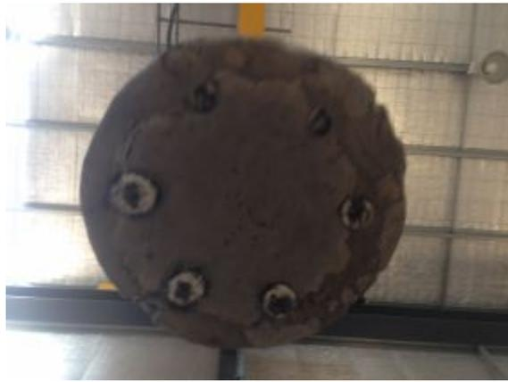
Figure 4.10: Longitudinal bars extruding from the base.
