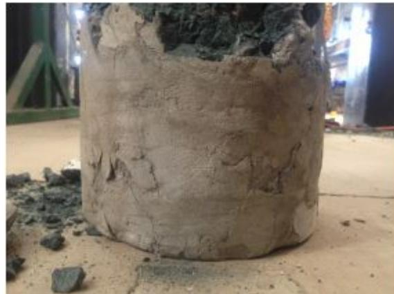
Figure 4.11: Cracking of the patched area.
