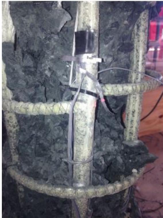
Figure 4.12: Shear failure of the C1-100 specimen.
