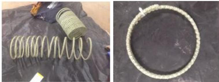
Figure 3.2: The spiral and circular ties used as transverse reinforcement.
