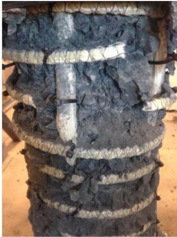
Figure 4.21: core crushing of the S1-50 specimen.
