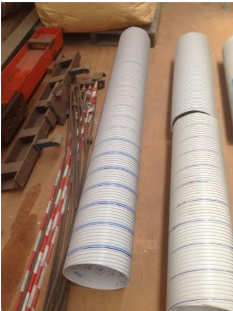
Figure 3.9: The formworks used for casting the specimens.
