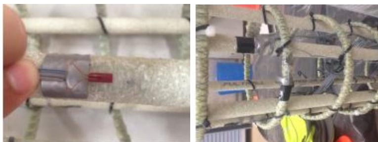
Figure 3.7: The attachment of the internal strain gauges.
