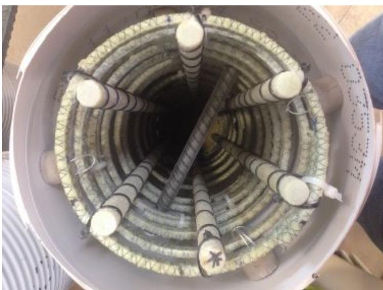
Figure 3.10: The internal configuration of each specimen.
