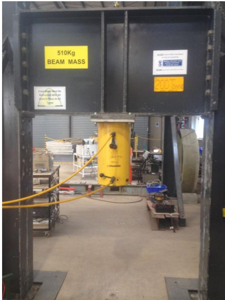
Figure C.1: The 2000kN hydraulic jack used.
