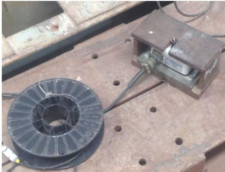
Figure C.7: The stringpot used to measure deflection.
