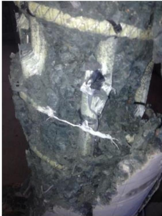
Figure 4.30: The buckling of the longitudinal bars.
