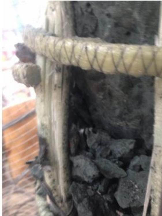
Figure 4.16: Splitting of the longitudinal bars and separation of circular ties for the C1-100 specimen.
