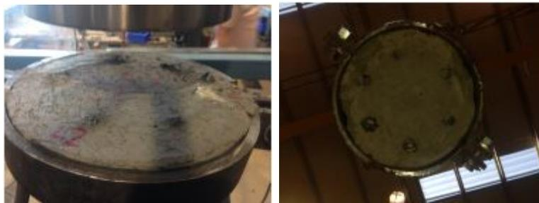
Figure 4.25: The extrusion of longitudinal bars of the specimen S1-50 from the top of the specimen (left) as well as the base (right).
