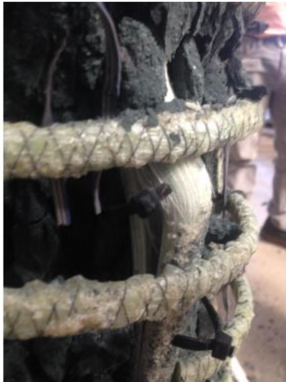
Figure 4.9: Bending of the longitudinal bars.
