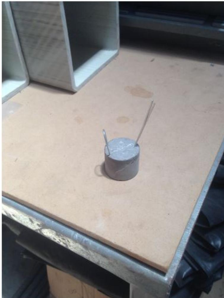
Figure 3.8: The concrete spacers.
