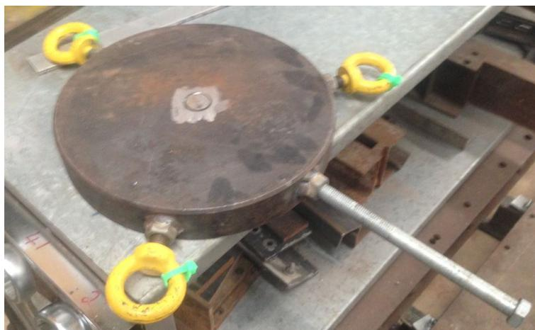
Figure C.2: The circular plate used to evenly distribute the load.
