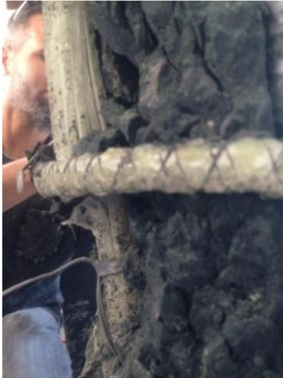
Figure 4.31: The splitting of the vertical bars.
