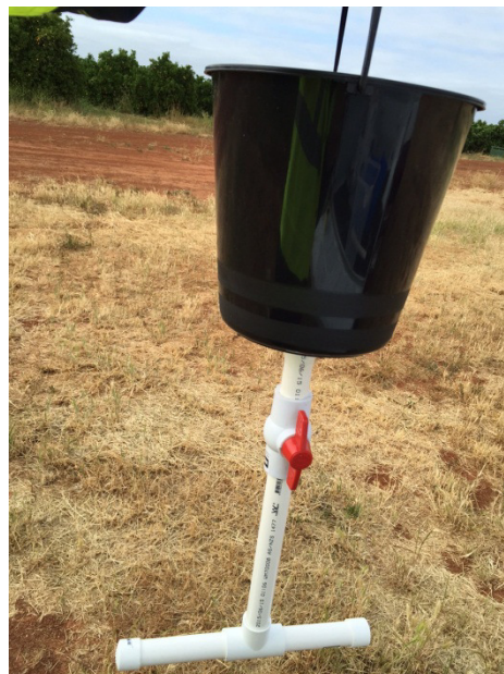
Figure 11 – 9L bucket, PVC pipework and ball valve used to apply stormwater over soil media within container.
