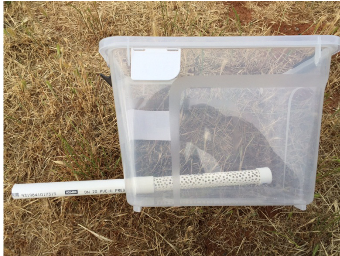
Figure 10 – 18L Container with porous PVC pipe at bottom used for Experimentation
