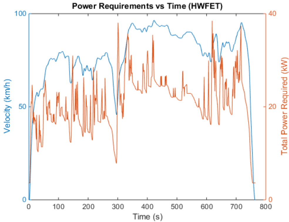
Figure 5.7: Total Power requirement vs time for HWFET cycle
