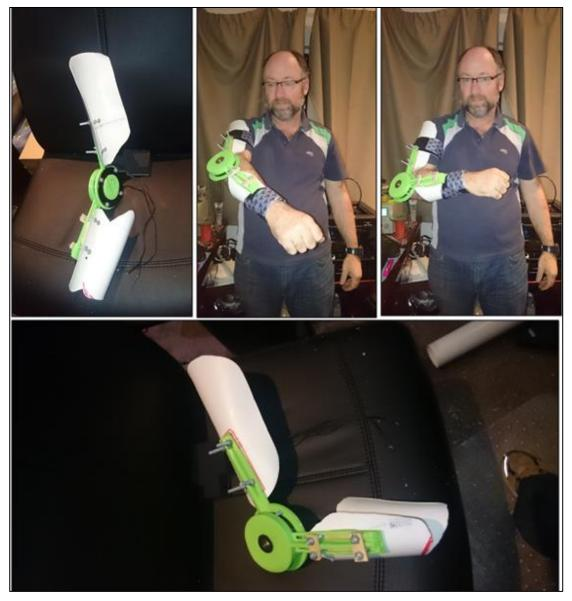
Figure 6-47: Initial PVC Splint
