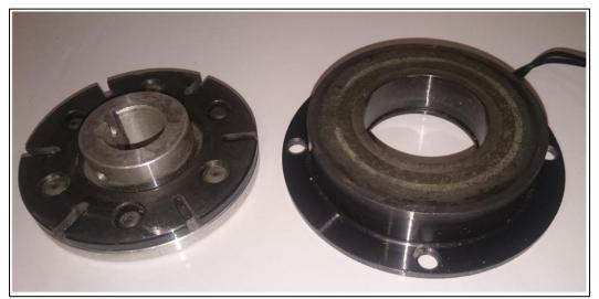
Figure 5-15: Electromagnetic Brake Pictured Apart
