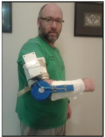
Figure 6-50: DSD with Electronic Box Secured with Velcro
