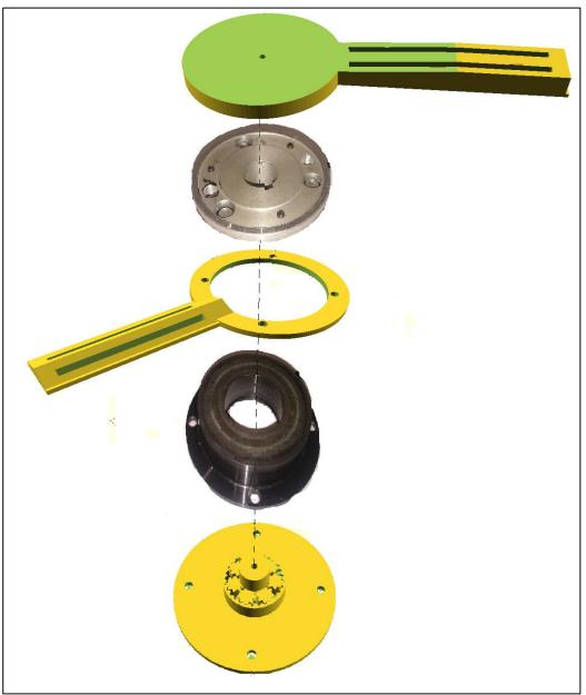
Figure 5-21: Exploded View of initial 3D Parts Design
