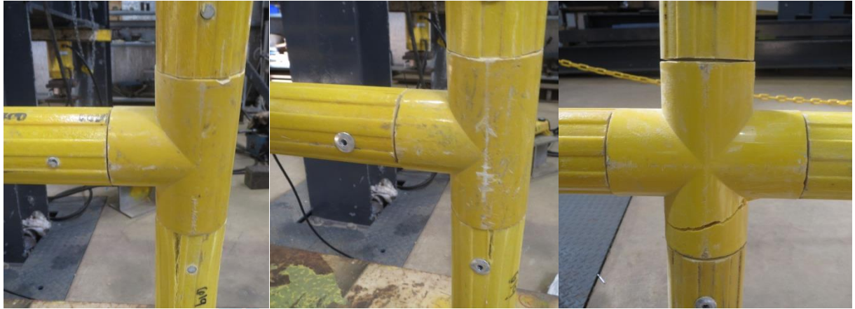
(a) Failure of the GFRP tube at side post
