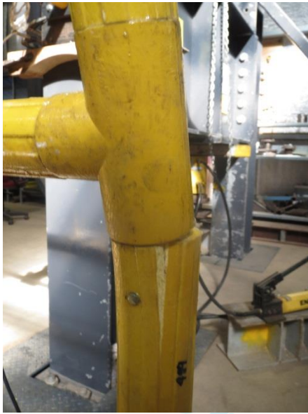
(a) Failure of FRP profile (side post)
