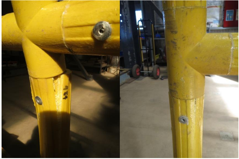
(b) Failure of FRP profile (middle and end posts)
