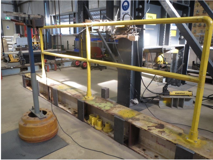
Figure 6: Test of GFRP guardrails loaded to the post (specimen GTP)
