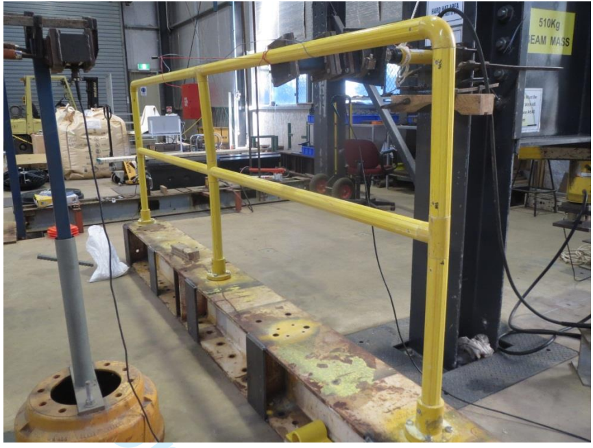
Figure 7: Test of GFRP guardrails loaded to the member (specimen GTM)
