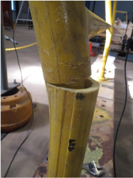
(a) Failure of joint (side post)
