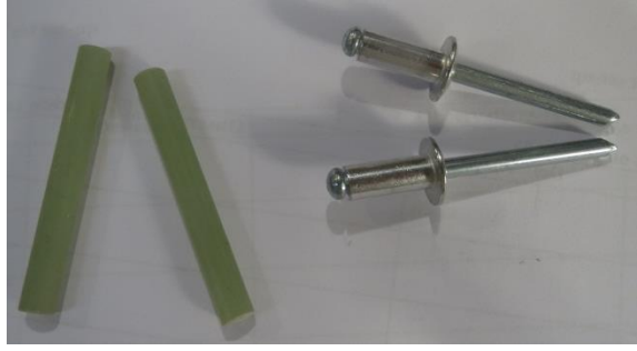
Figure 4: Polypin (left) and rivets (right) fasteners for the composite guardrail
