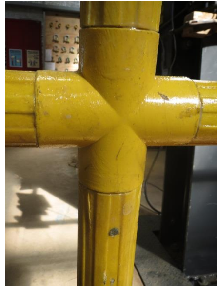
(b) Failure of FRP profile (middle post)
