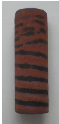
Figure 1: (a) A post-combustion trace on a hollow cylinder. (b) A running spinning wave solution of Eq. (1) (five successive shapes) evolved from a random initial condition [1].
