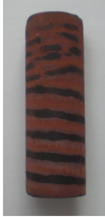
(a) A post-combustion trace left by the spinning solid flame on a hollow cylinder; courtesy of A.G. Strunina (see also similar photos and discussions in [2, 10]).
