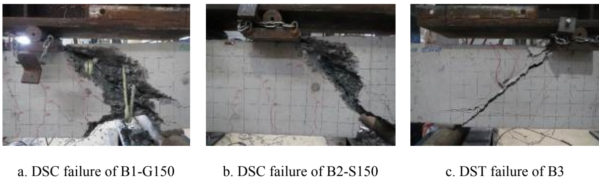
Figure 5 Failure mode of the tested beams.
