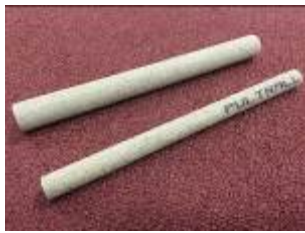
Figure 2 Sand-coated GFRP bars.
