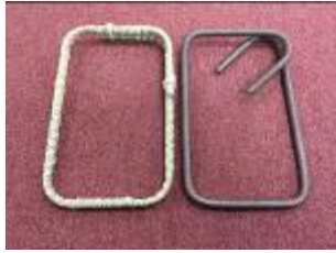
Figure 1 GFRP and steel stirrups.
