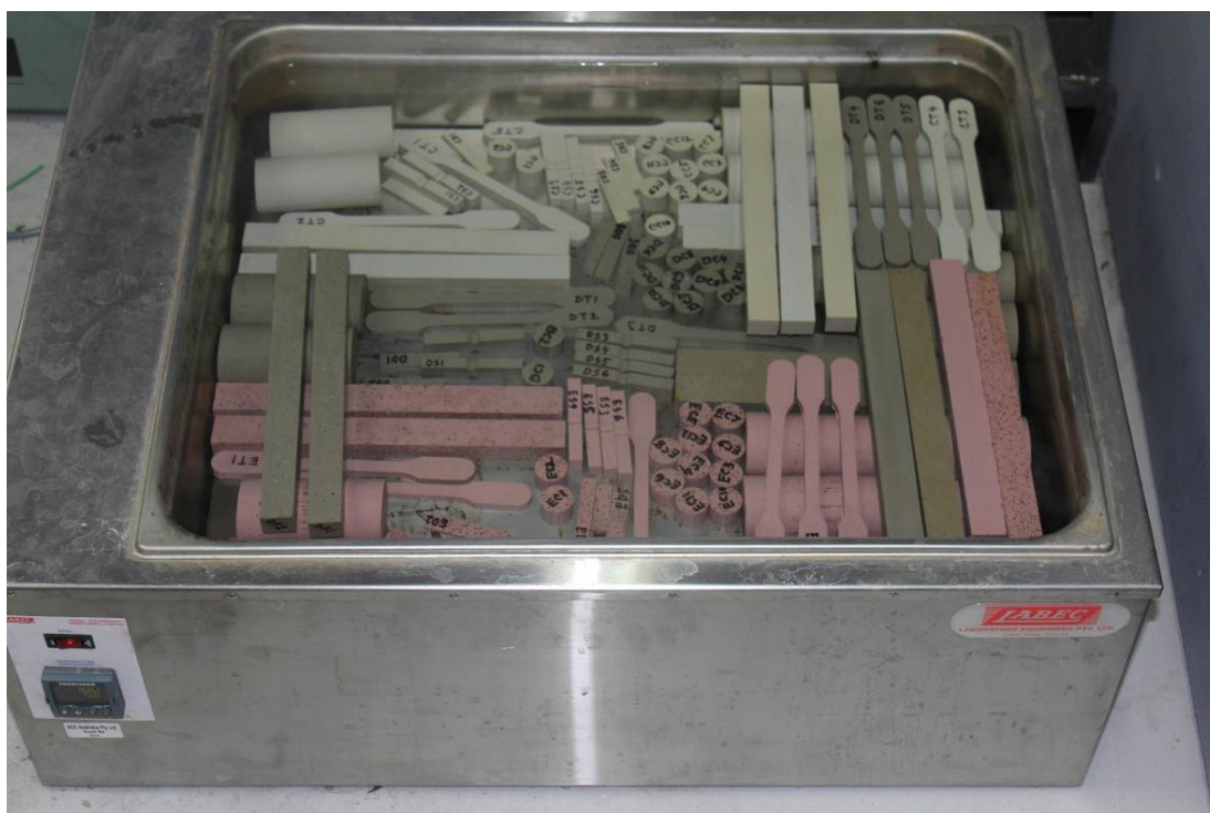
Figure 4.2 Grout specimens being conditioned at the water bath
