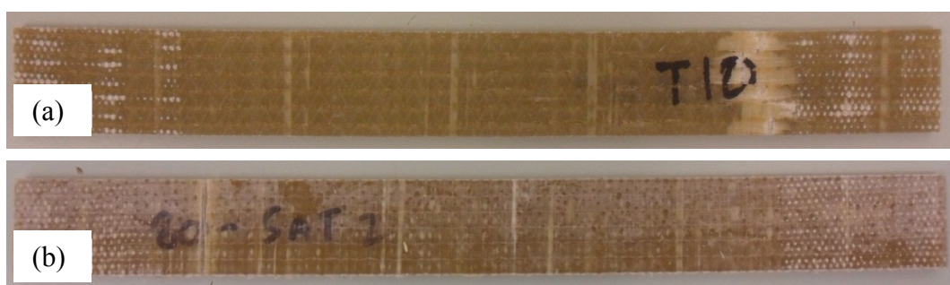
Figure 5.8 Typical tensile failure pattern of conditioned LT laminate specimens; (a) HWC – 1000 specimens, (b) HWC – 3000 specimens
