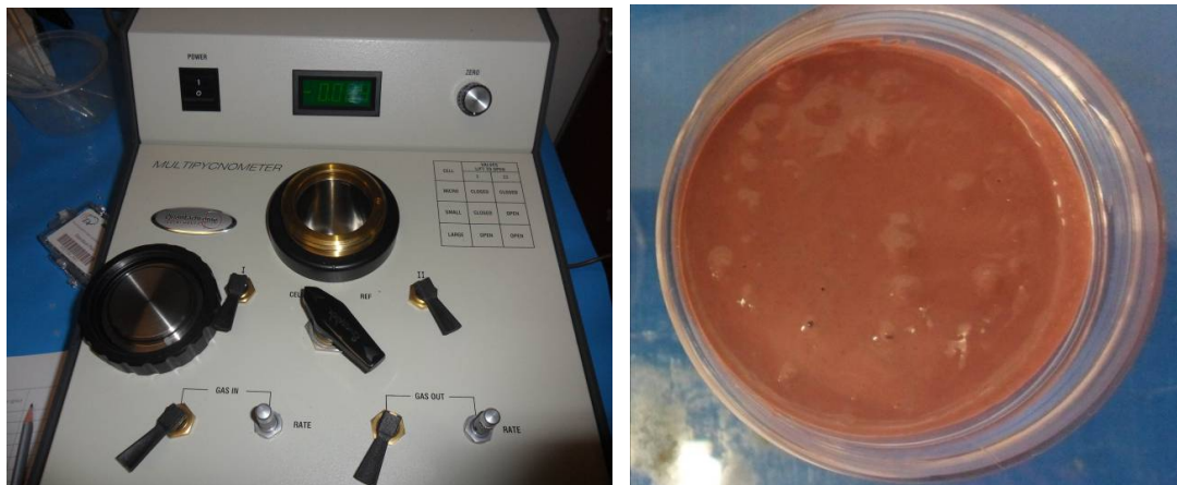
Figure A. 1 Shrinkage test apparatus and grout samples
