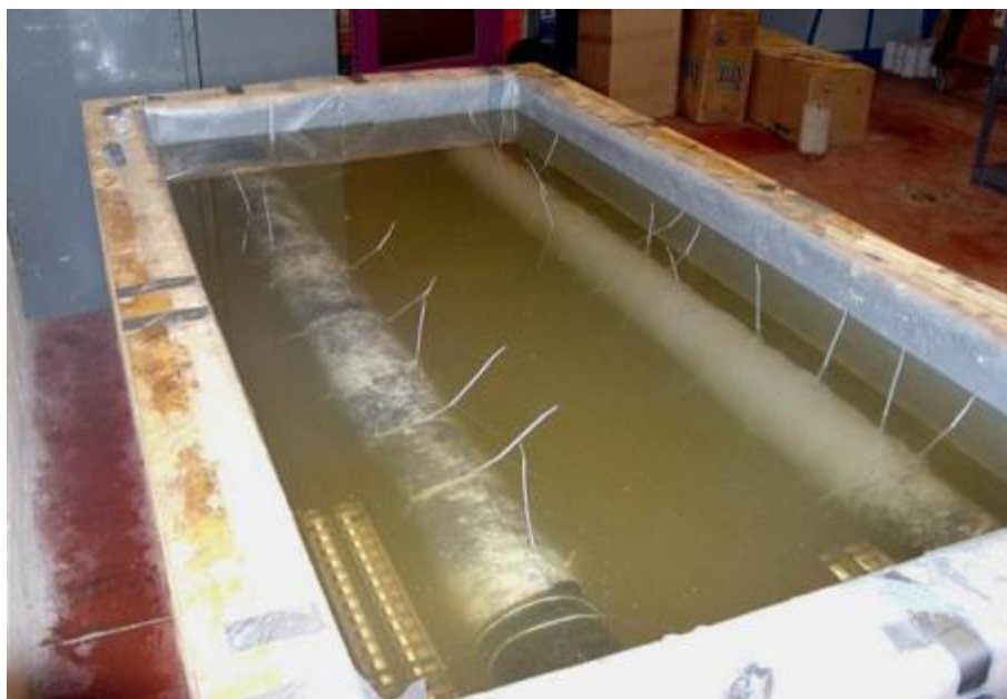
Figure 2.2 Flexible CFRP-wrapped specimens being cured under saltwater conditions (Seica & Packer 2007)
