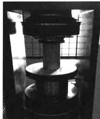
Figure 1. Uniaxial compressive test
